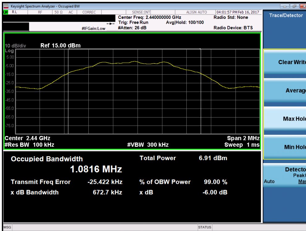
Plot 7-2. 6dB Bandwidth Plot (Bluetooth (LE) – Ch. 19)
