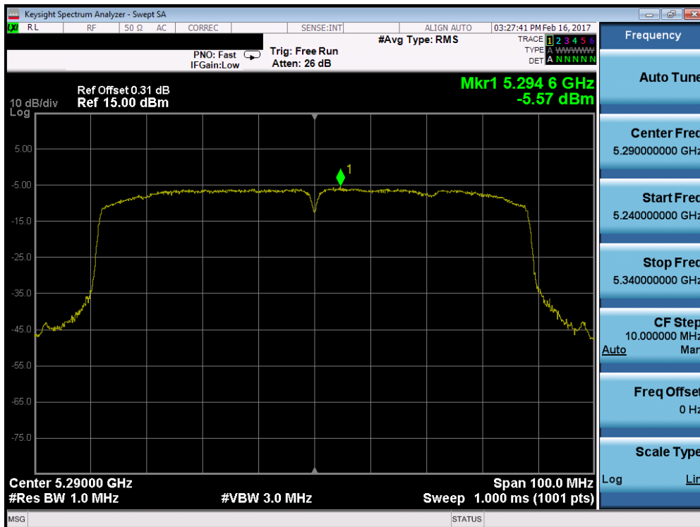
Plot 7-55. Power Spectral Density Plot (80MHz BW 802.11ac (UNII Band 2A) – Ch. 58)
