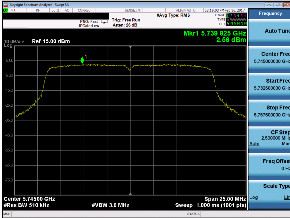
Plot 7-69. Power Spectral Density Plot (20MHz BW 802.11n (UNII Band 3) – Ch. 149)
