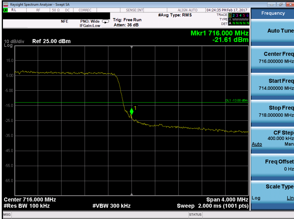
Plot 7-123. Upper Band Edge Plot (Band 12 – 5.0MHz QPSK – RB Size 25)
