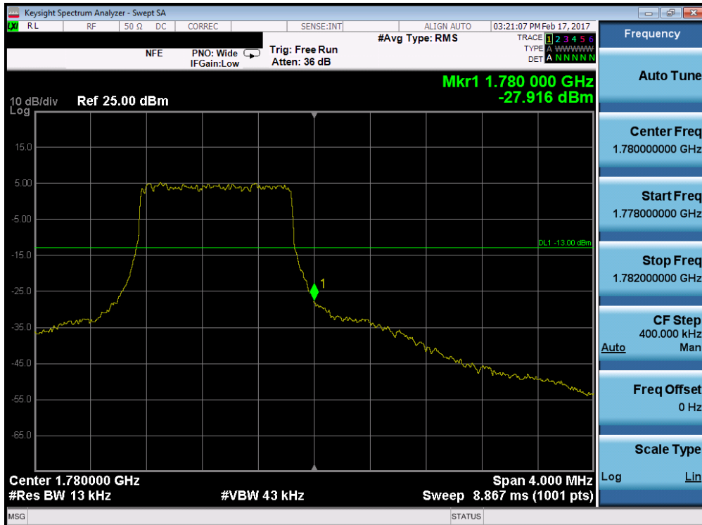
Plot 7-136. Upper Band Edge Plot (Band 4/66 – 1.4MHz QPSK – RB Size 6)
