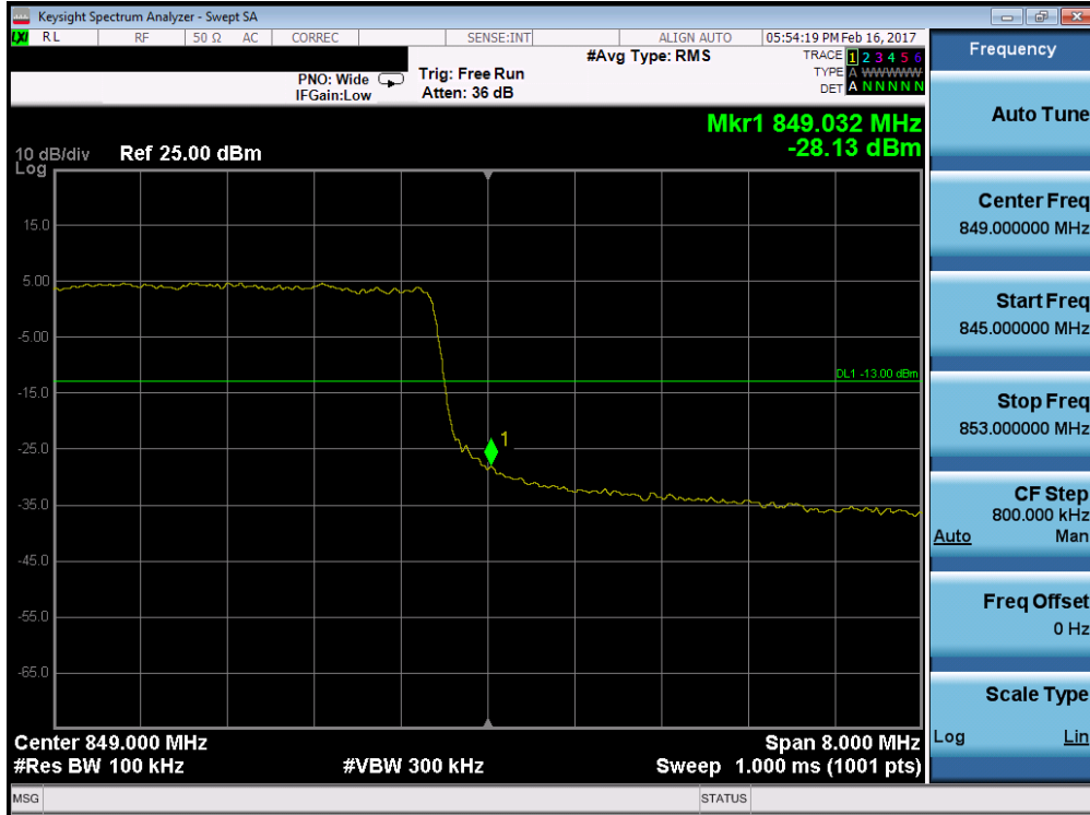
Plot 7-133. Upper Band Edge Plot (Band 5 – 10.0MHz QPSK – RB Size 50)
