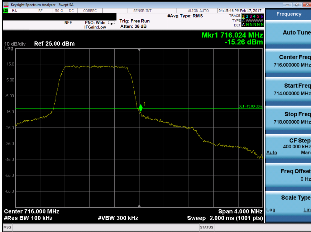
Plot 7-119. Upper Band Edge Plot (Band 12 – 1.4MHz QPSK – RB Size 6)
