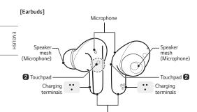
$\label{eq:Microphone} Microphone$  \*Make sure that the charging terminal is not soiled with foreign substance.
