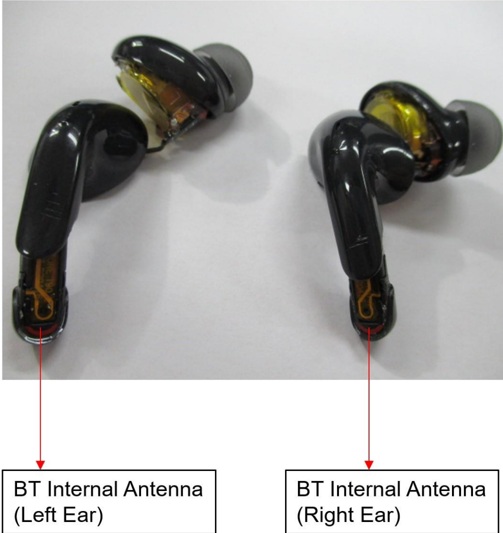
Figure E-1 Antenna Location (Rear Side View)
