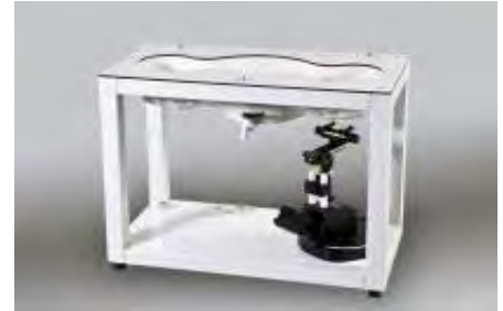
Figure E.5.1 SAM Twin Phantom
