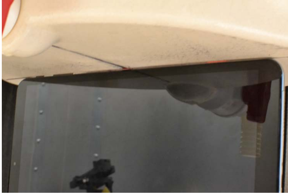
SAR Test Setup Photo 5 – Right Edge at 0 mm
