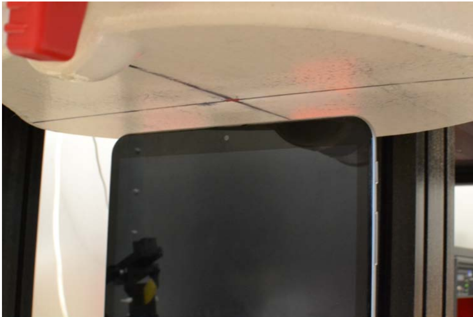
SAR Test Setup Photo 3 – Top Edge at 15 mm
