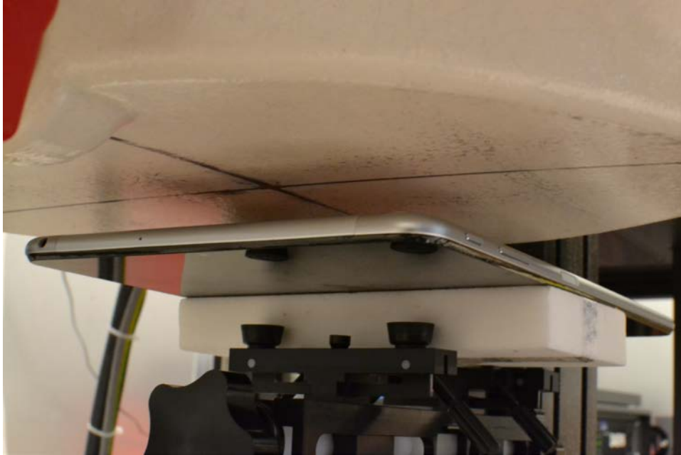
SAR Test Setup Photo 1 – Back Side at 15 mm
