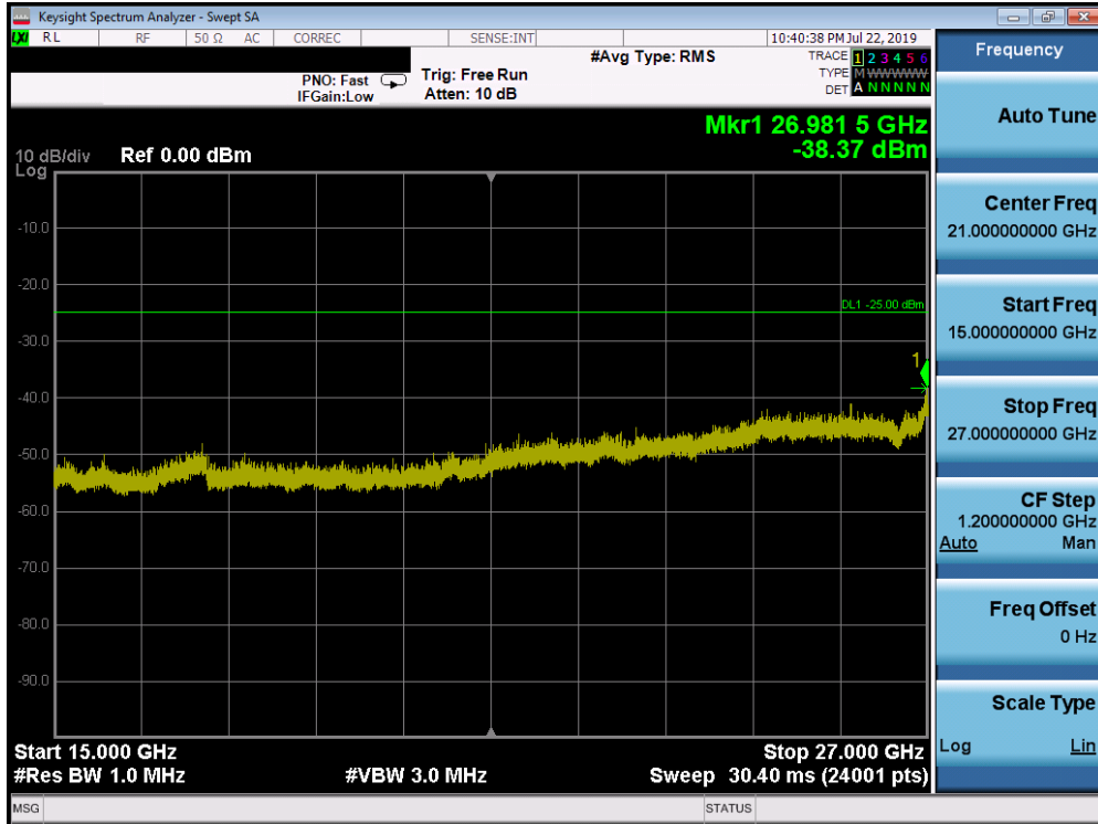
Plot 7-171. Conducted Spurious Plot (Band 41 PC3 - 20.0MHz QPSK - RB Size 1, RB Offset 0 - Low Channel)
