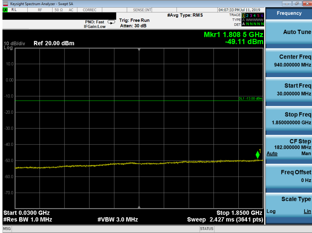
Plot 7-157. Conducted Spurious Plot (Band 25/2- 20.0MHz QPSK - RB Size 1, RB Offset 0 - High Channel)
