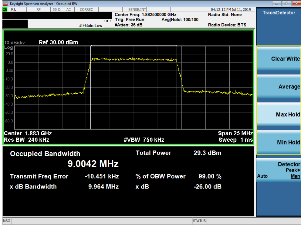
Plot 7-74. Occupied Bandwidth Plot (Band 25/2 - 10.0MHz 16-QAM - Full RB Configuration)
