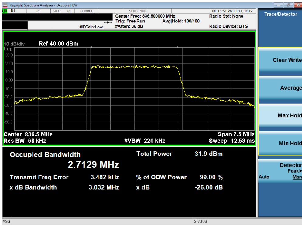
Plot 7-34. Occupied Bandwidth Plot (Band 26/5 - 3.0MHz QPSK - Full RB Configuration)
