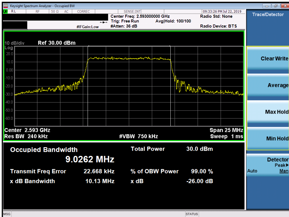
Plot 7-99. Occupied Bandwidth Plot (Band 41 PC3 - 10.0MHz 64-QAM - Full RB Configuration)
