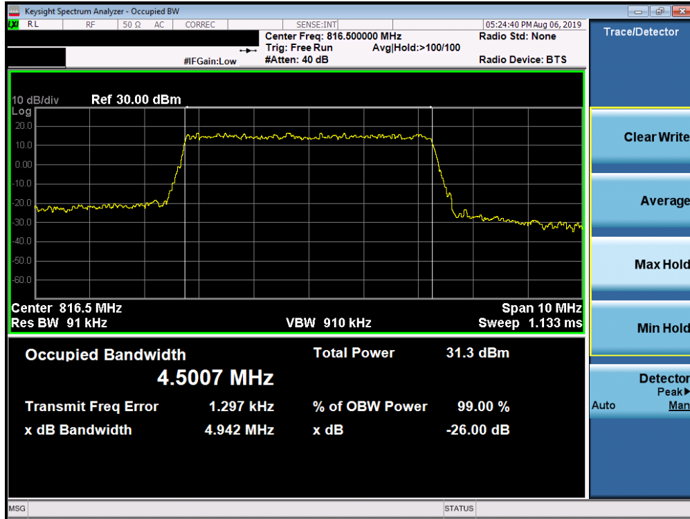
Plot 7-9. Occupied Bandwidth Plot (LTE Band 26, 5MHz 64-QAM – RB Size 25– Low Channel)
