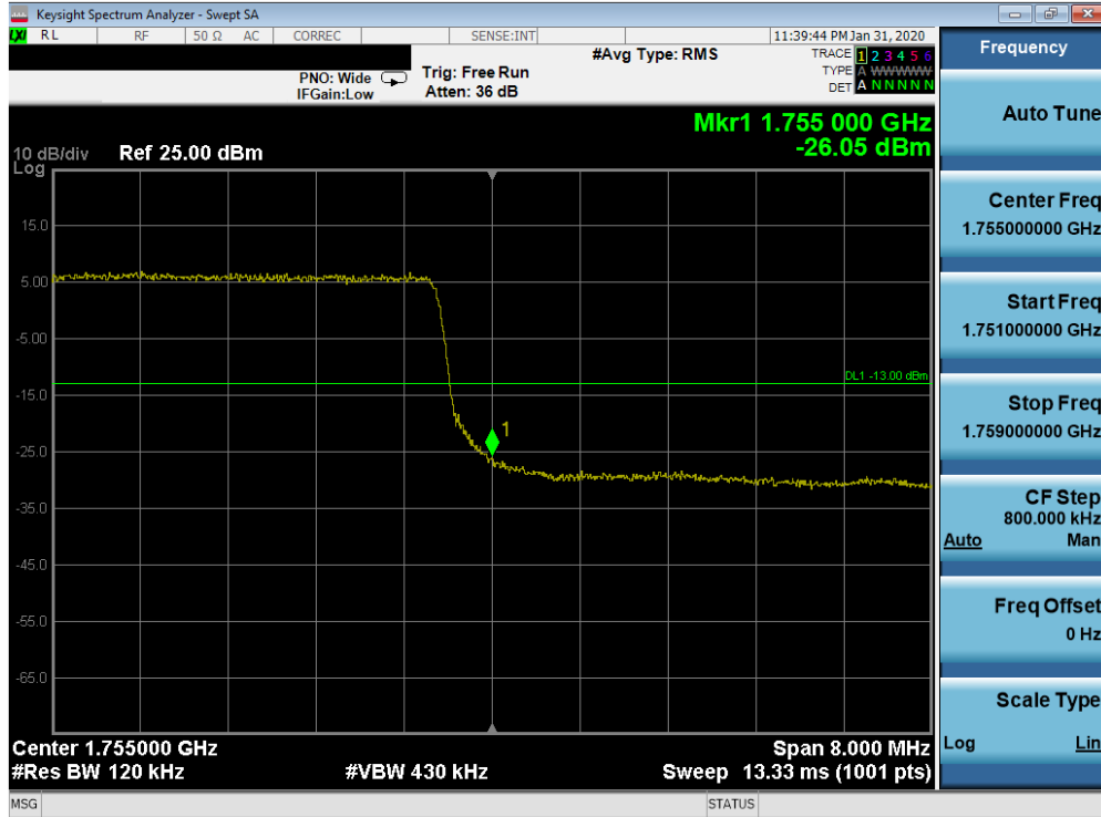
Plot 7-205. Upper Band Edge Plot (Band 4 - 10.0MHz QPSK - Full RB Configuration)
