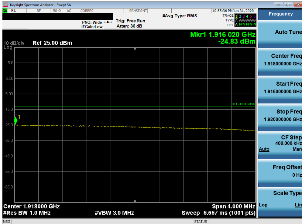
Plot 7-256. Upper Extended Band Edge Plot (Band 25 - 20.0MHz QPSK - Full RB Configuration)
