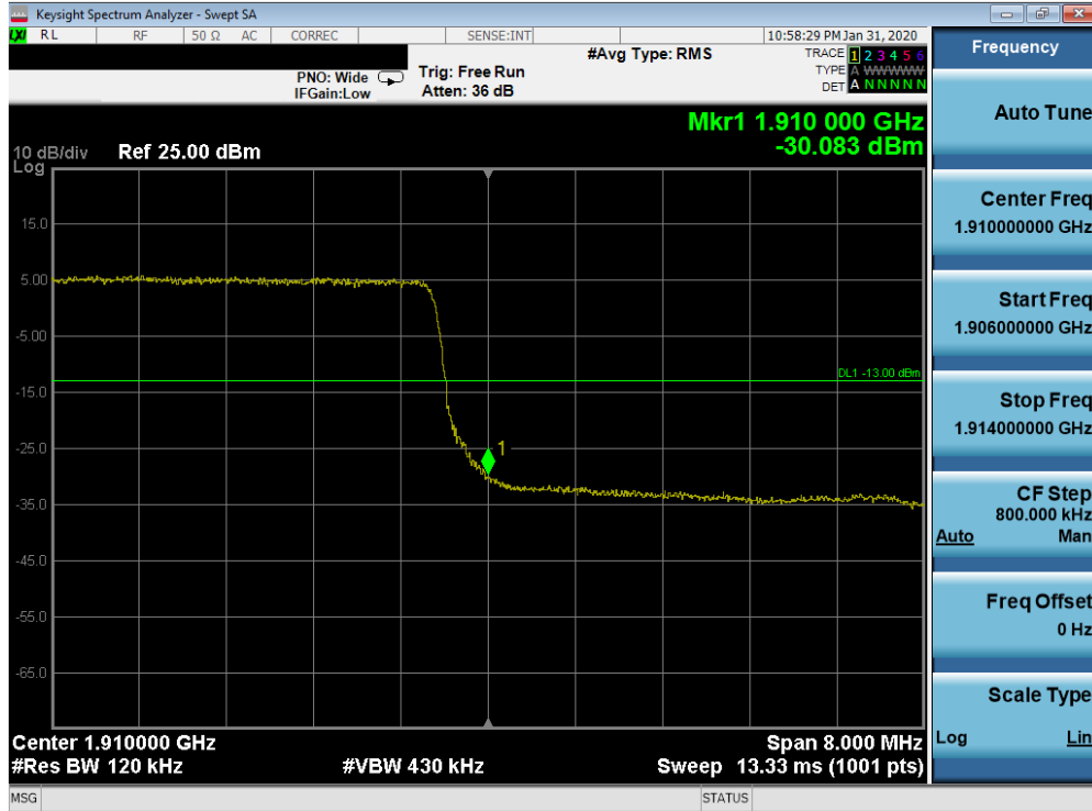
Plot 7-241. Upper Band Edge Plot (Band 2 - 10.0MHz QPSK - Full RB Configuration)
