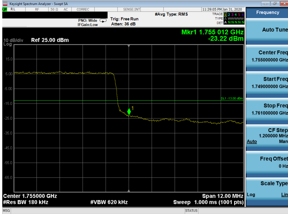
Plot 7-211. Upper Band Edge Plot (Band 4 - 15.0MHz QPSK - Full RB Configuration)
