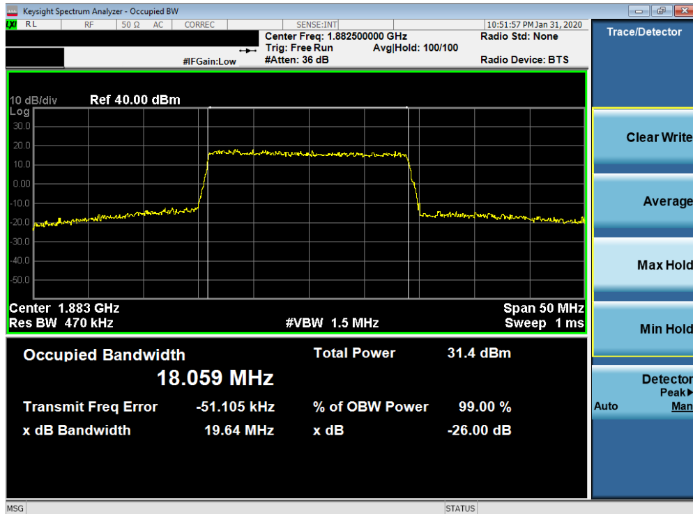
Plot 7-81. Occupied Bandwidth Plot (Band 25/2 - 20.0MHz 64-QAM - Full RB Configuration)
