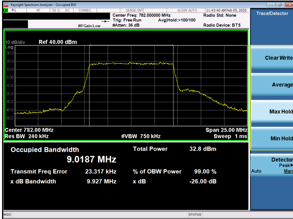
Plot 7-29. Occupied Bandwidth Plot (Band 13 - 10.0MHz 16-QAM - Full RB Configuration)
