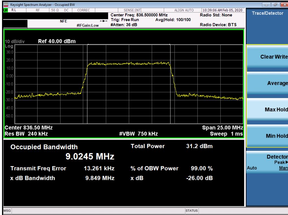
Plot 7-41. Occupied Bandwidth Plot (Band 26/5 - 10.0MHz 16-QAM - Full RB Configuration)
