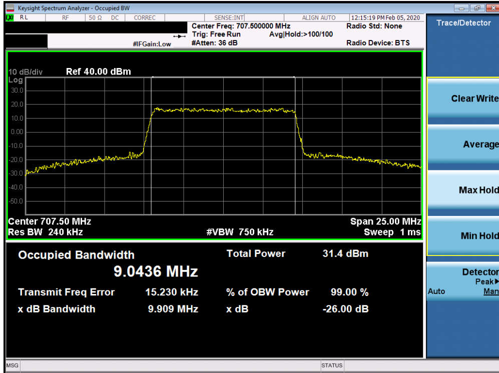
Plot 7-23. Occupied Bandwidth Plot (Band 12 - 10.0MHz 16-QAM - Full RB Configuration)
