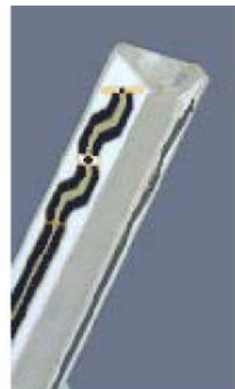
Figure 3.3 Probe Thick-Film Technique
