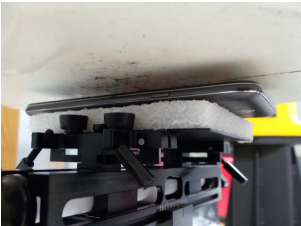
SAR Test Setup Photo 6: Front Side at 10 mm
