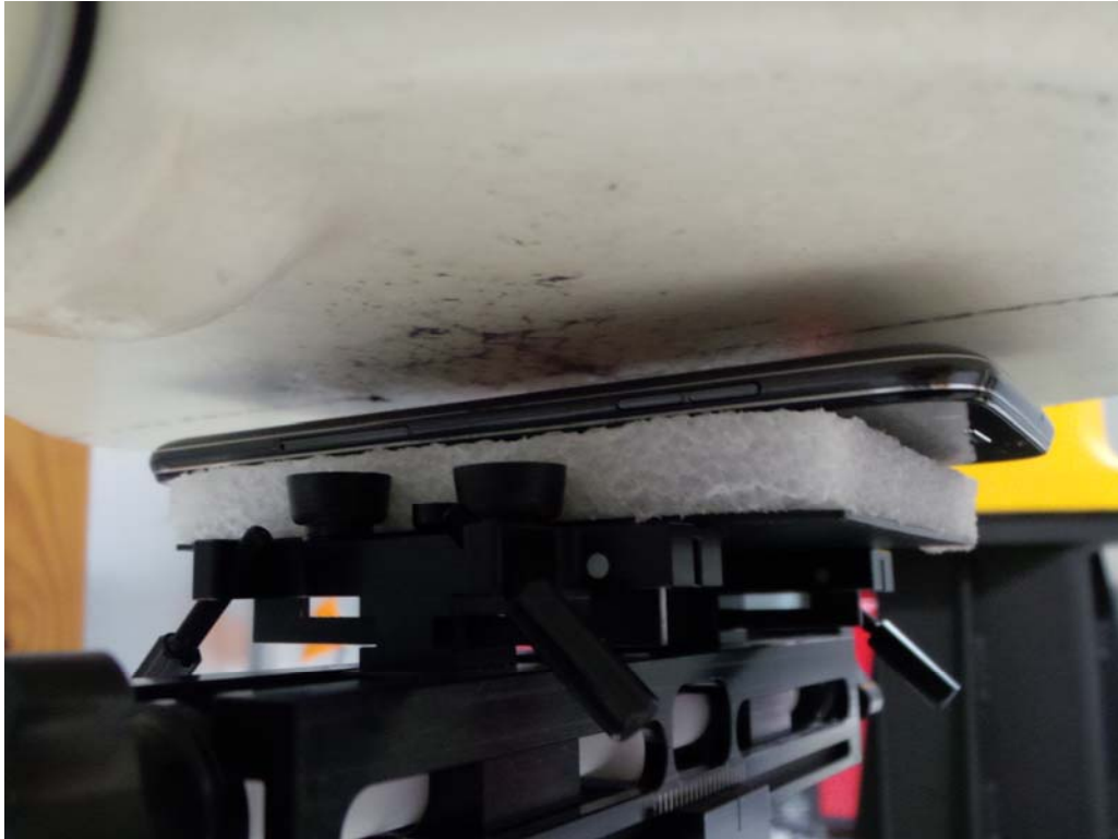
SAR Test Setup Photo 5: Back Side at 10 mm
