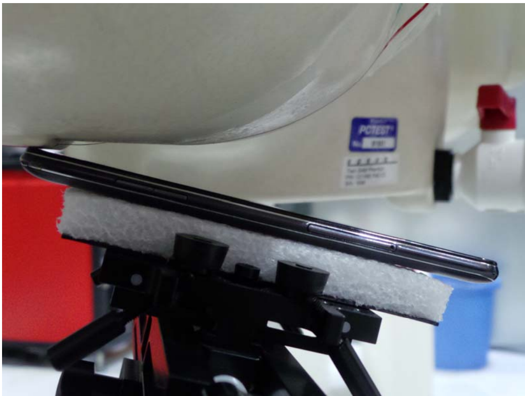
SAR Test Setup Photo 2: Right Tilt
