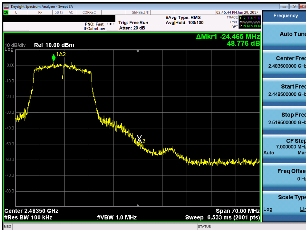
Plot 7-22. Band Edge Plot (802.11g – Ch. 11)
