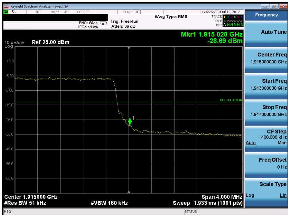
Plot 7-179. Upper Band Edge Plot (Band 25 - 5.0MHz QPSK - RB Size 25)
