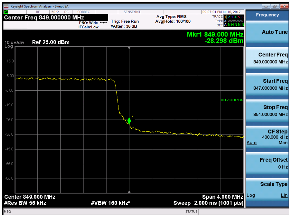
Plot 7-135. Upper Band Edge Plot (Band 5/26 - 5.0MHz QPSK - RB Size 25)
