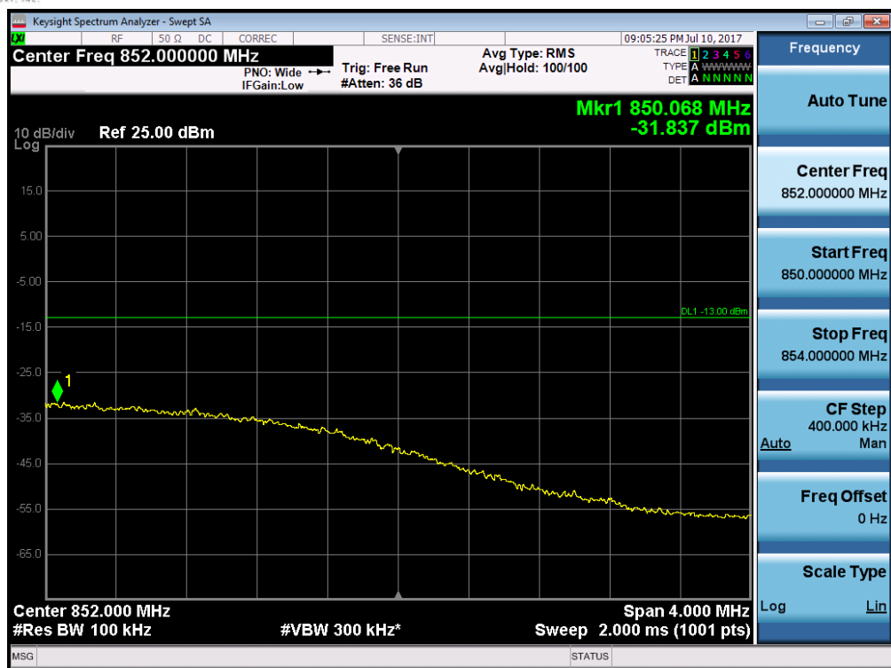
Plot 7-136. Upper Extended Band Edge Plot (Band 5/26 – 5.0MHz QPSK – RB Size 25)
