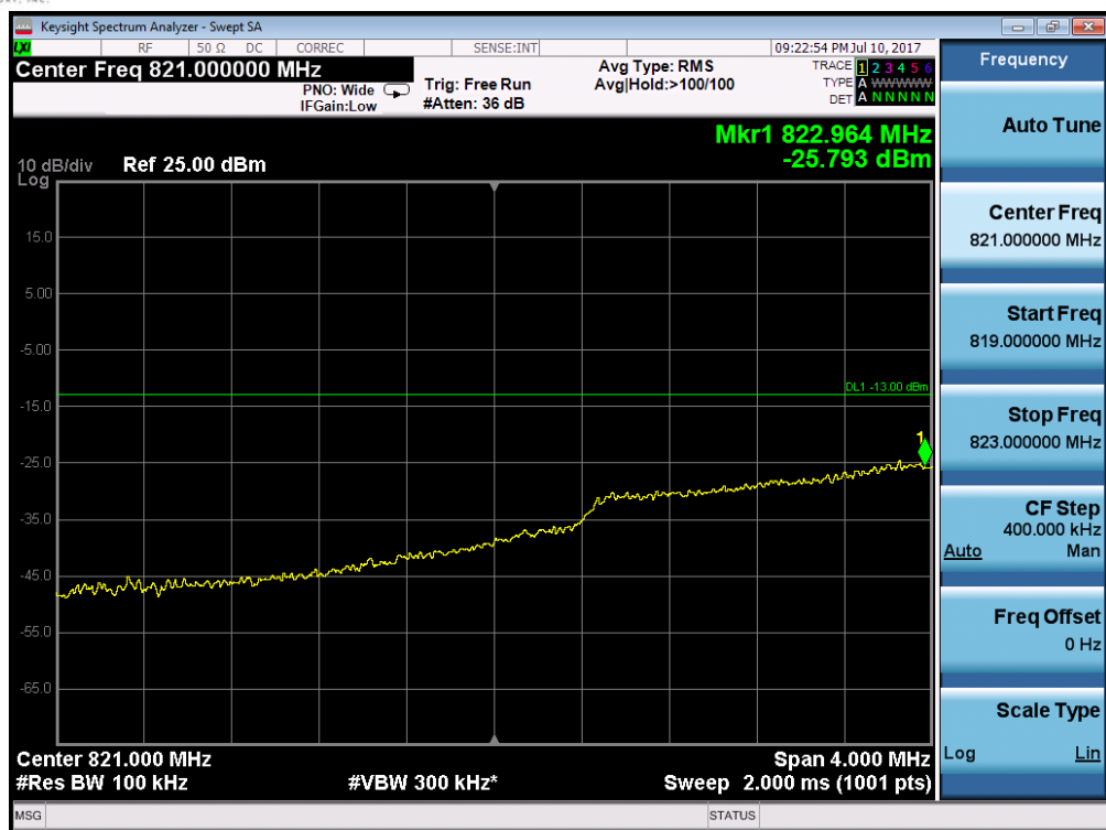
Plot 7-130. Lower Extended Band Edge Plot (Band 5/26 - 3.0MHz QPSK - RB Size 15)
