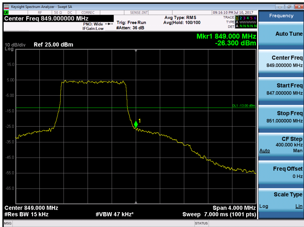
Plot 7-127. Upper Band Edge Plot (Band 5/26 – 1.4MHz QPSK – RB Size 6)
