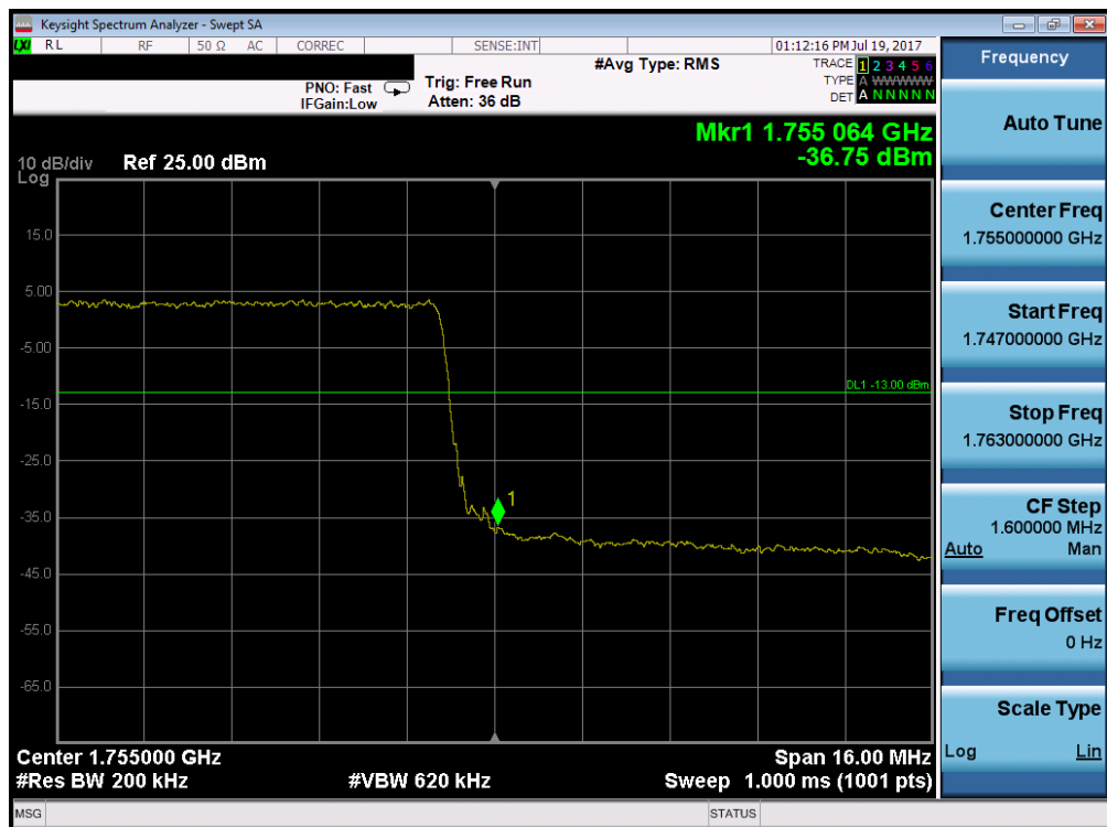
Plot 7-167. Upper Band Edge Plot (Band 4 – 20.0MHz QPSK – RB Size 100)
