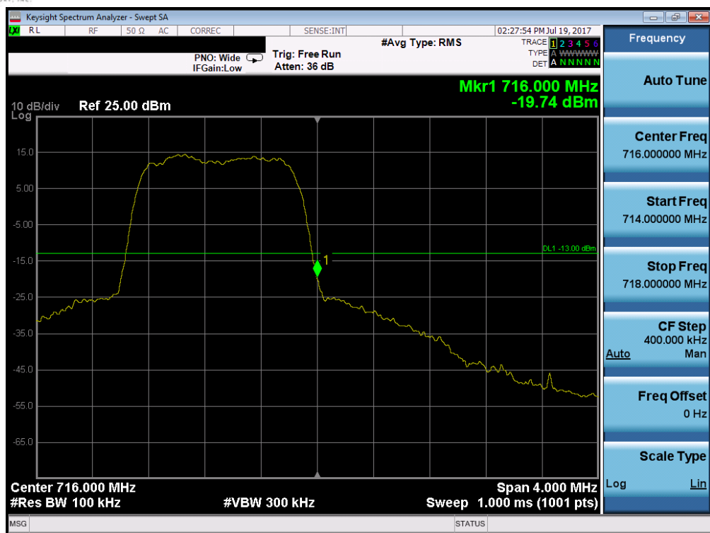
Plot 7-110. Upper Band Edge Plot (Band 12 – 1.4MHz QPSK – RB Size 6)
