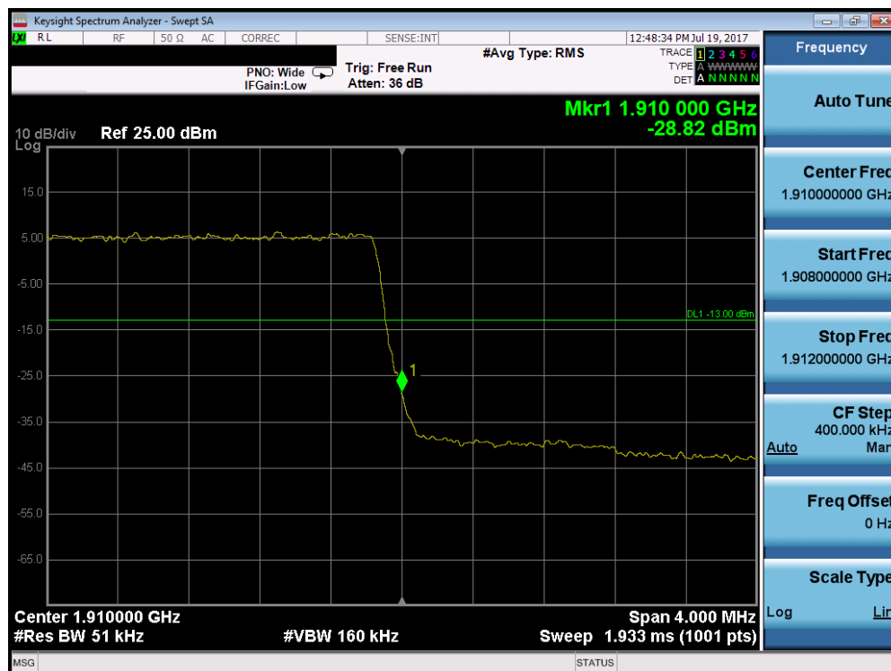
Plot 7-195. Upper Band Edge Plot (Band 2 – 3.0MHz QPSK – RB Size 15)
