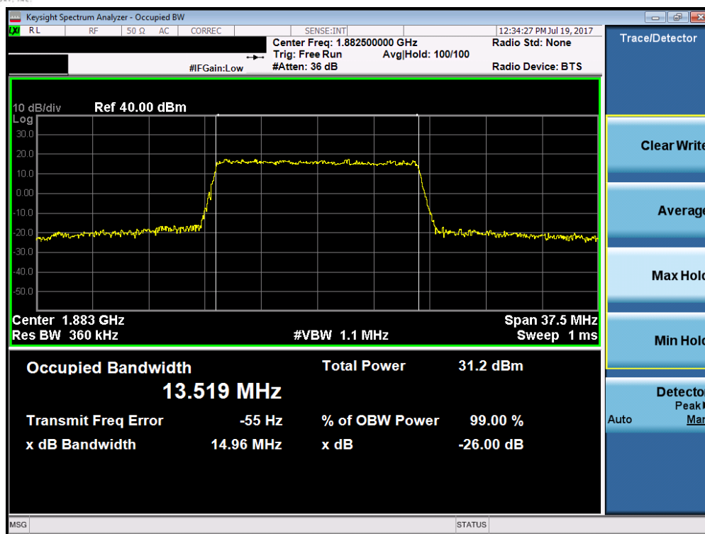
Plot 7-43. Occupied Bandwidth Plot (Band 2/25 – 15.0MHz QPSK – RB Size 75)
