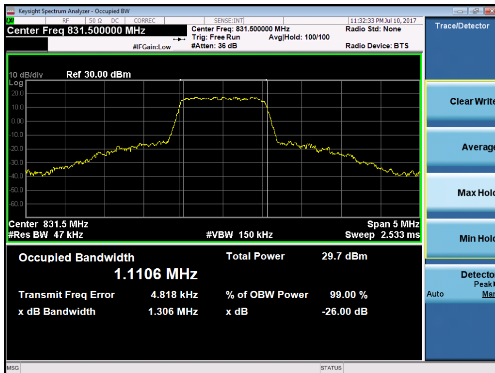
Plot 7-14. Occupied Bandwidth Plot (Band 26/5 – 1.4MHz 16-QAM – RB Size 6)
