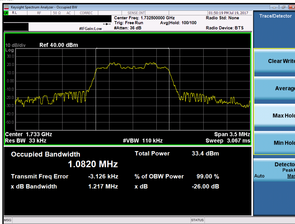
Plot 7-23. Occupied Bandwidth Plot (Band 4 – 1.4MHz QPSK – RB Size 6)
