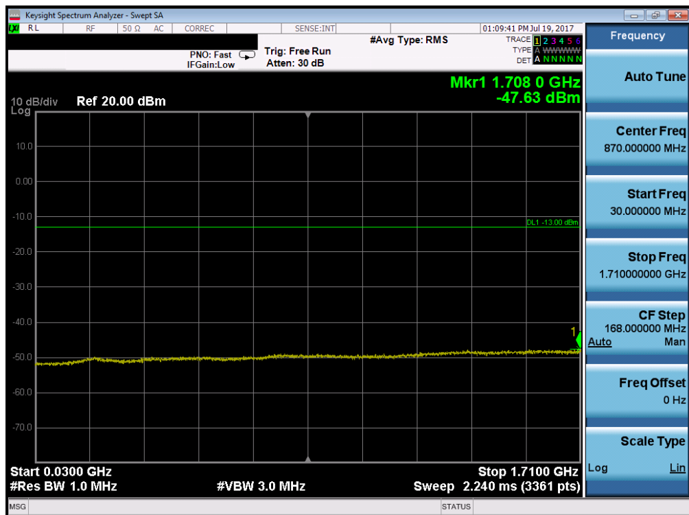
Plot 7-88. Conducted Spurious Plot (Band 4 – 15.0MHz QPSK – RB Size 1, RB Offset 0 – High Channel)
