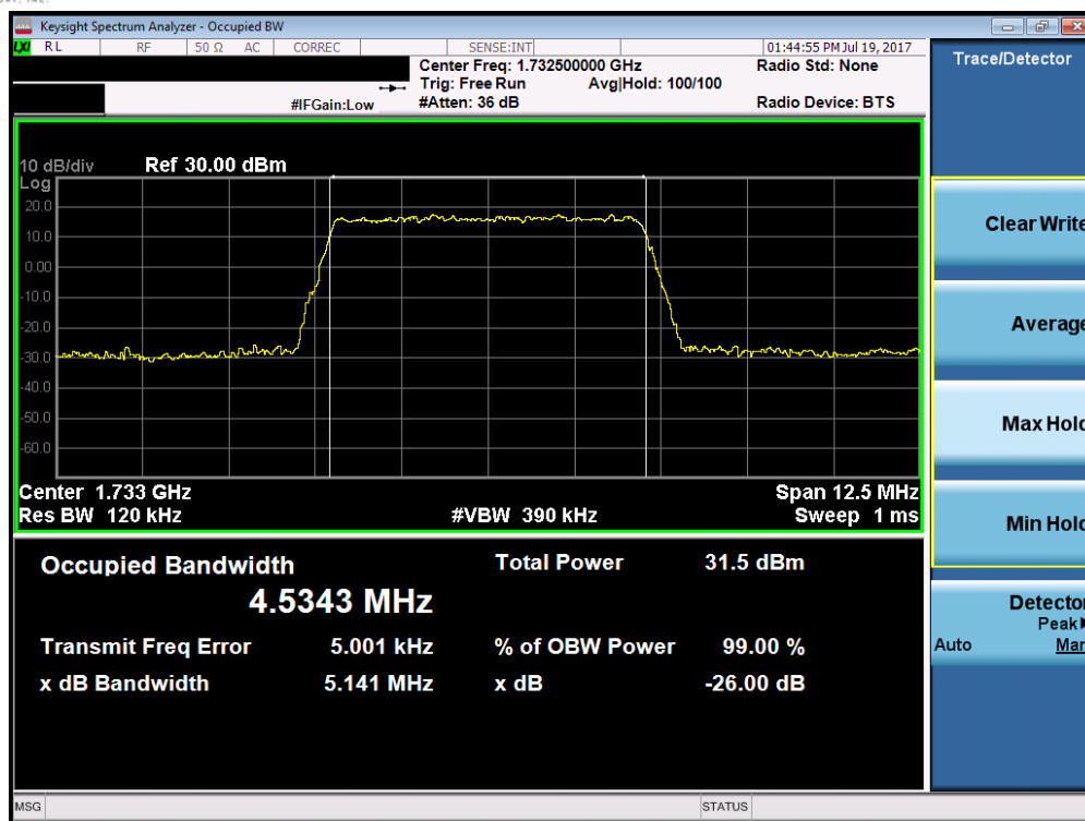
Plot 7-27. Occupied Bandwidth Plot (Band 4 – 5.0MHz QPSK – RB Size 25)
