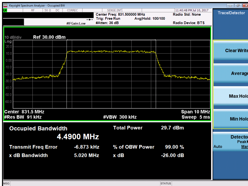
Plot 7-18. Occupied Bandwidth Plot (Band 26/5 – 5.0MHz 16-QAM – RB Size 25)
