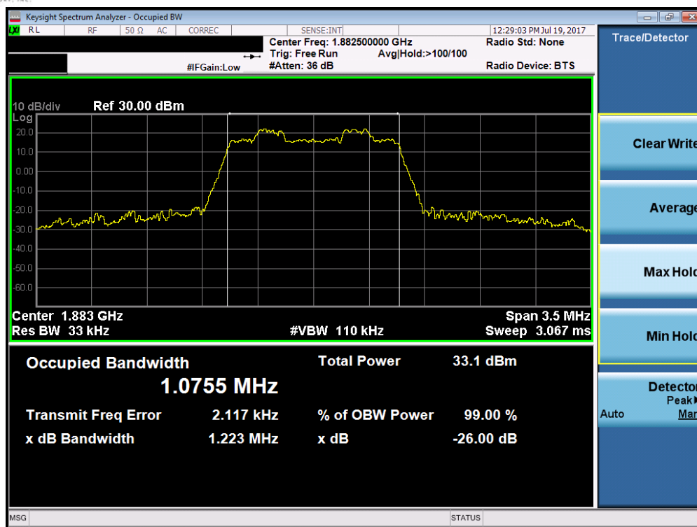
Plot 7-35. Occupied Bandwidth Plot (Band 2/25 – 1.4MHz QPSK – RB Size 6)
