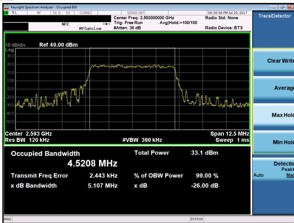
Plot 7-47. Occupied Bandwidth Plot (Band 41 – 5.0MHz QPSK – RB Size 25)
