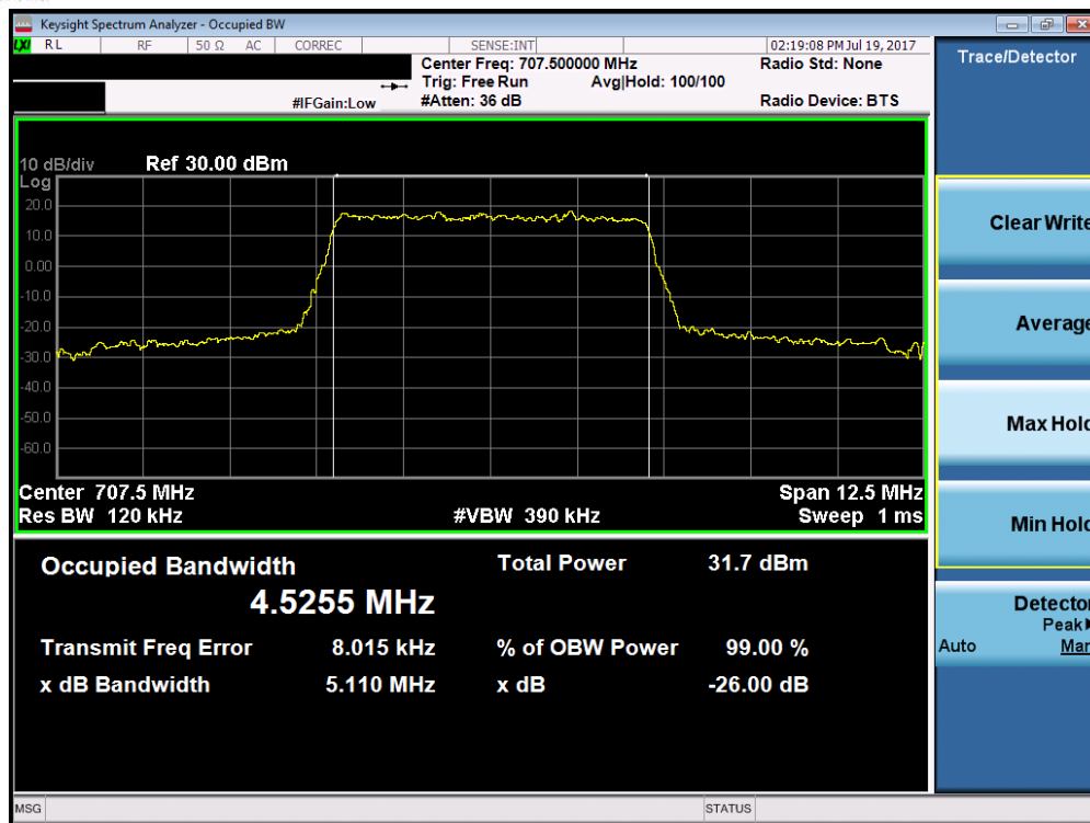
Plot 7-5. Occupied Bandwidth Plot (Band 12 – 5.0MHz QPSK – RB Size 25)
