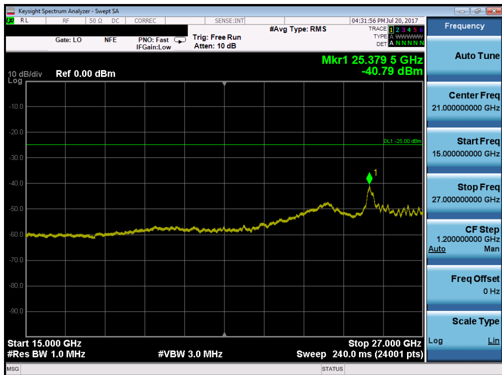
Plot 7-102. Conducted Spurious Plot (Band 41 – 15.0MHz QPSK – RB Size 1, RB Offset 0 – Low Channel)
