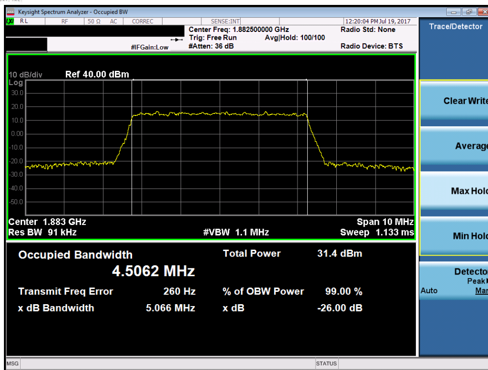
Plot 7-39. Occupied Bandwidth Plot (Band 2/25 - 5.0MHz QPSK - RB Size 25)
