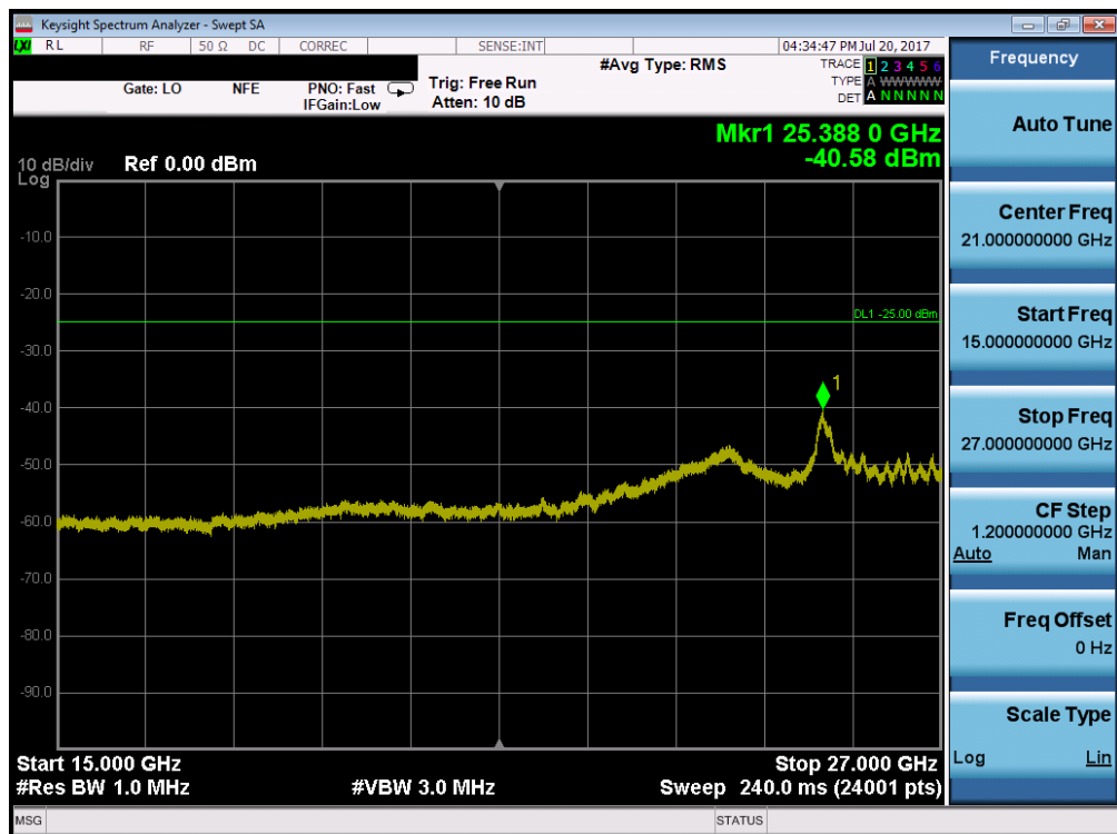
Plot 7-108. Conducted Spurious Plot (Band 41 – 15.0MHz QPSK – RB Size 1, RB Offset 0 – High Channel)
