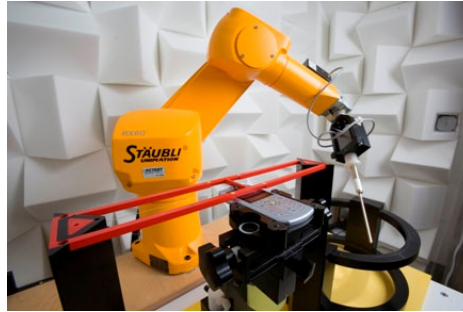
Figure 4-3 SPEAG Robotic System
