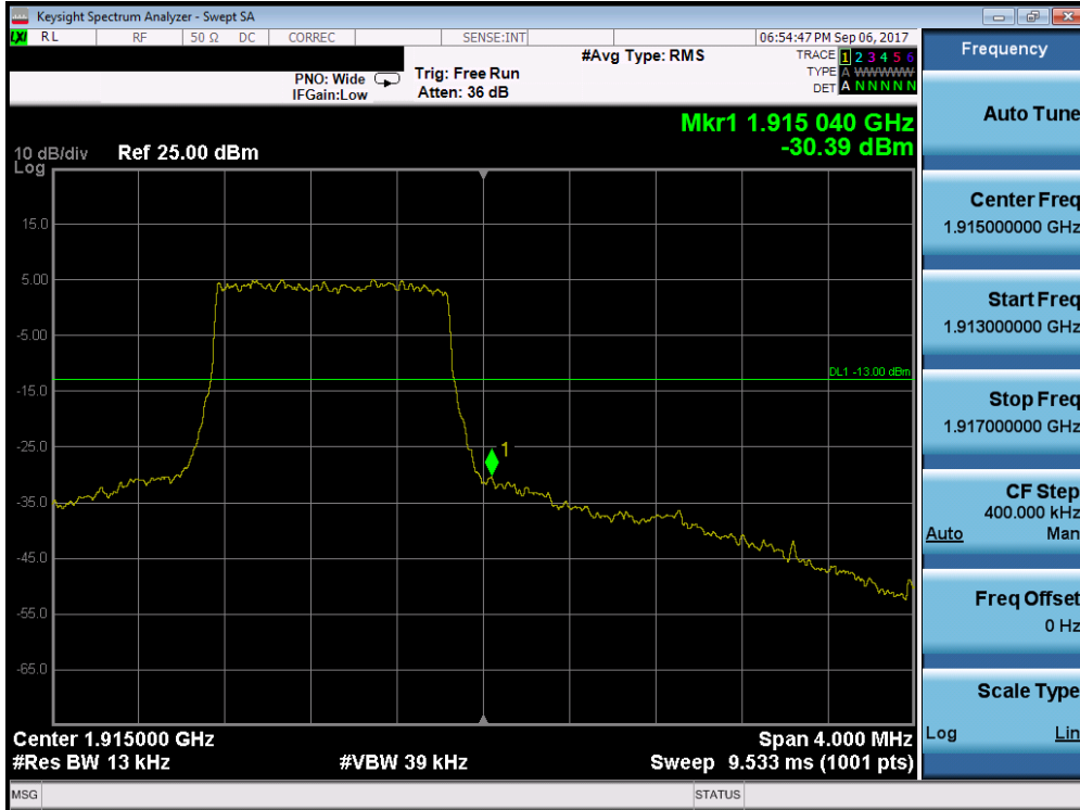
Plot 7-152. Upper Band Edge Plot (Band 25 – 1.4MHz QPSK - Full RB Configuration)
