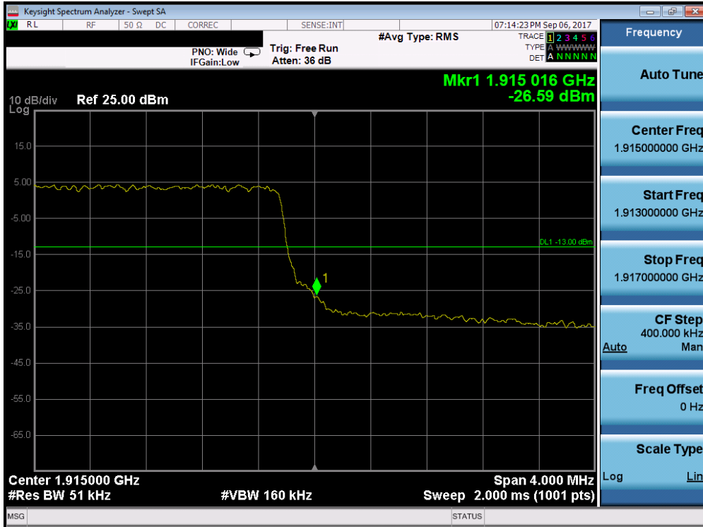
Plot 7-160. Upper Band Edge Plot (Band 25 - 5.0MHz QPSK - Full RB Configuration)
