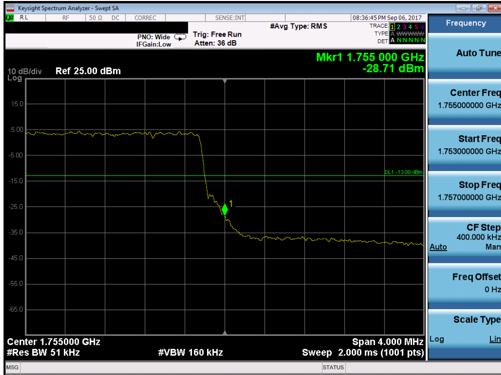
Plot 7-136. Upper Band Edge Plot (Band 4 - 5.0MHz QPSK - Full RB Configuration)
