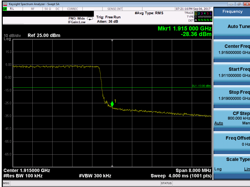
Plot 7-164. Upper Band Edge Plot (Band 25 - 10.0MHz QPSK - Full RB Configuration)
