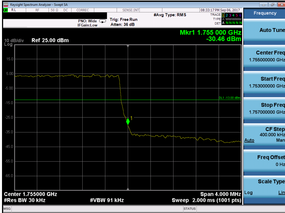
Plot 7-132. Upper Band Edge Plot (Band 4 - 3.0MHz QPSK - Full RB Configuration)
