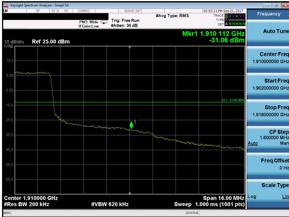
Plot 7-184. Upper Band Edge Plot (Band 2 – 20.0MHz QPSK - Full RB Configuration)
