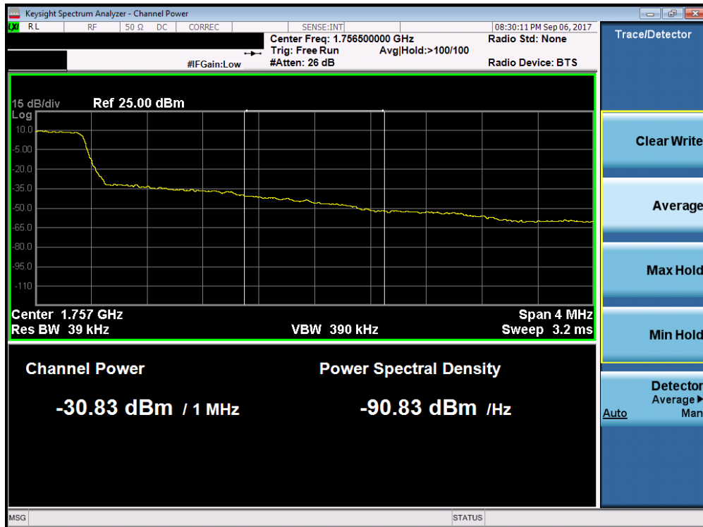
Plot 7-129. . Upper Extended Band Edge Plot (Band 4 – 1.4MHz QPSK - Full RB Configuration)
