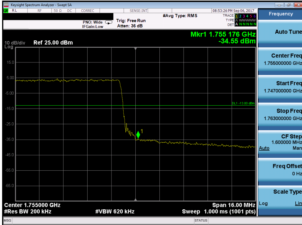
Plot 7-148. Upper Band Edge Plot (Band 4 - 20.0MHz QPSK - Full RB Configuration)
