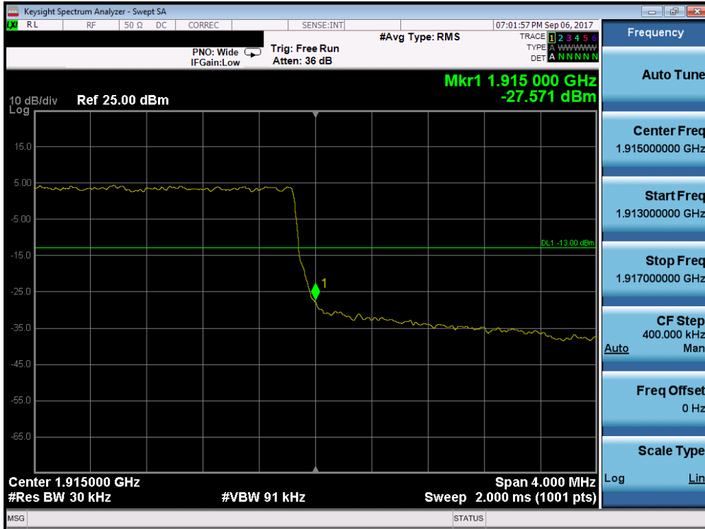
Plot 7-156. Upper Band Edge Plot (Band 25 - 3.0MHz QPSK - Full RB Configuration)
