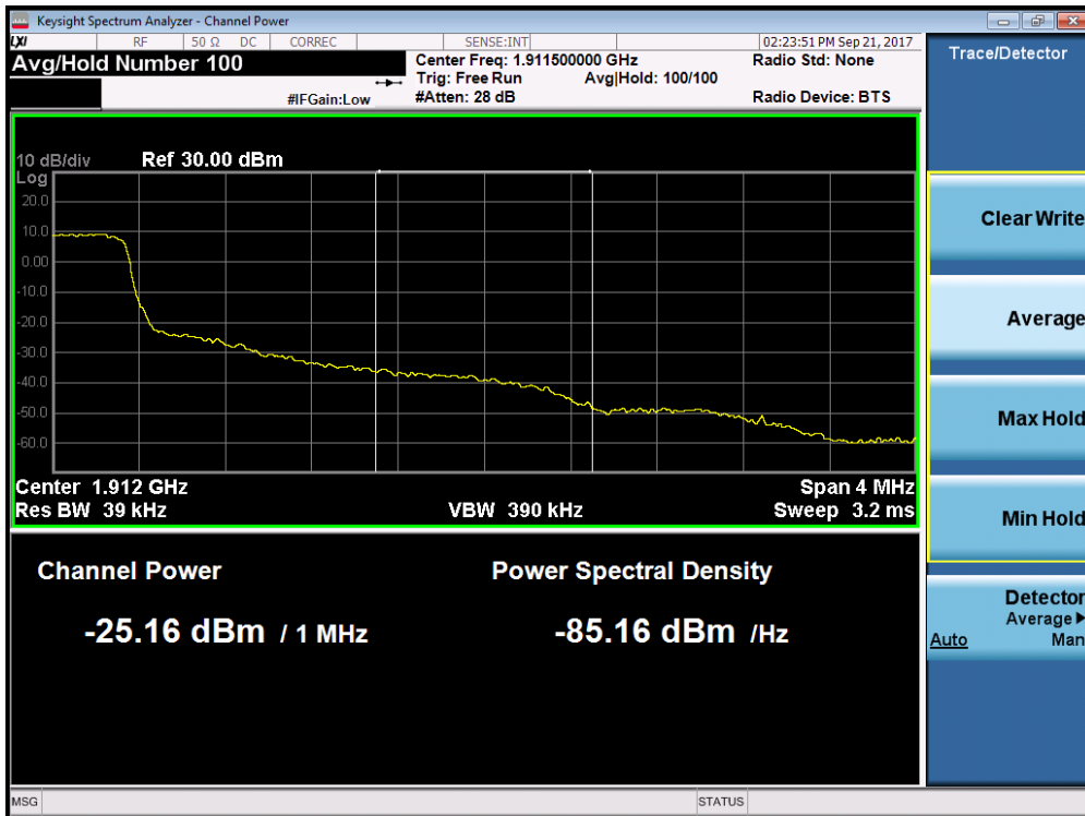
Plot 7-175. . Upper Extended Band Edge Plot (Band 2 – 1.4MHz QPSK - Full RB Configuration)
