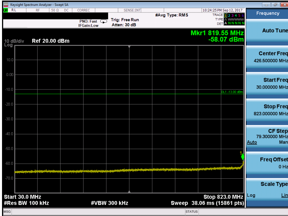
Plot 7-69. Conducted Spurious Plot (Band 26/5 - 10.0MHz QPSK - RB Size 1, RB Offset 0 - Low Channel)
