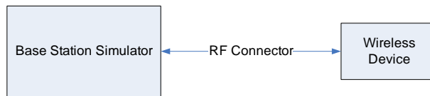
Figure 9-1 Power Measurement Setup
