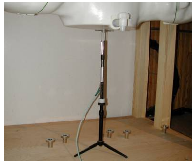
Figure 10-2 System Verification Setup Photo
