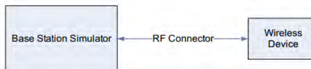
Figure 10.1 Power Measurement Setup
