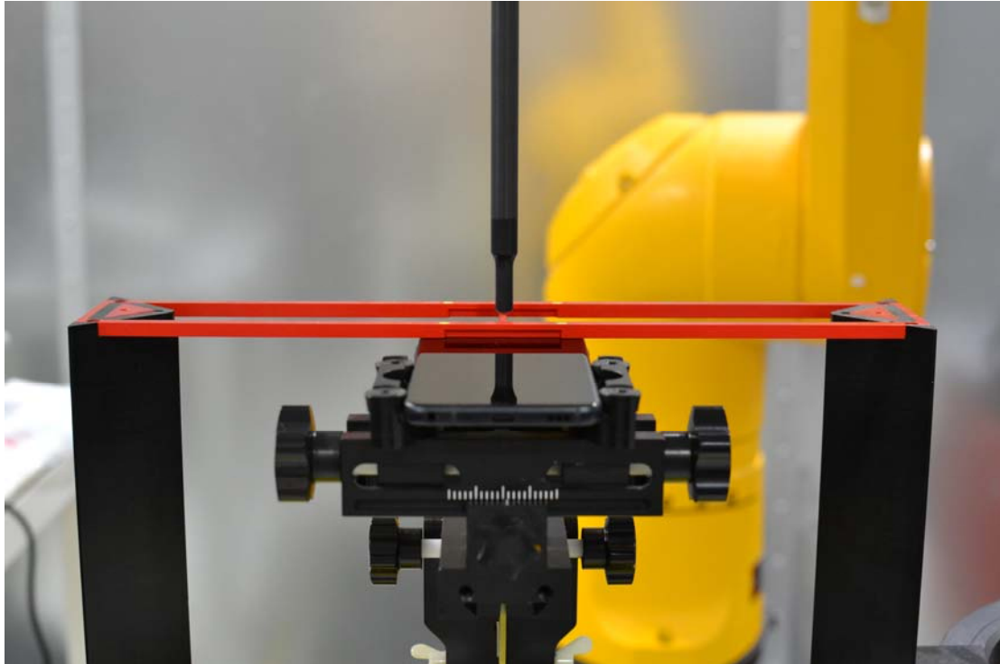
Figure 18-1 Ear Reference Point HAC Phantom Alignment
