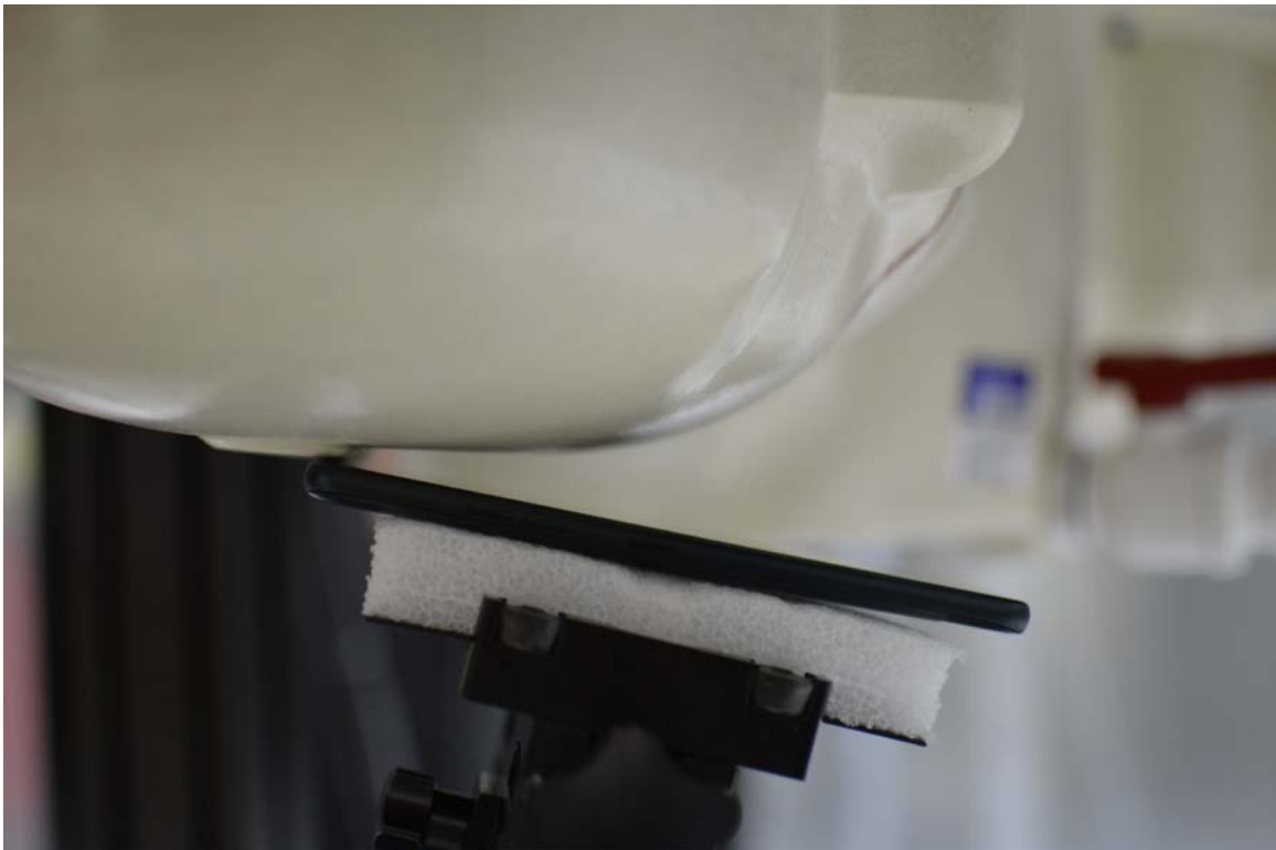
SAR Test Setup Photo 2 – Right Tilt
