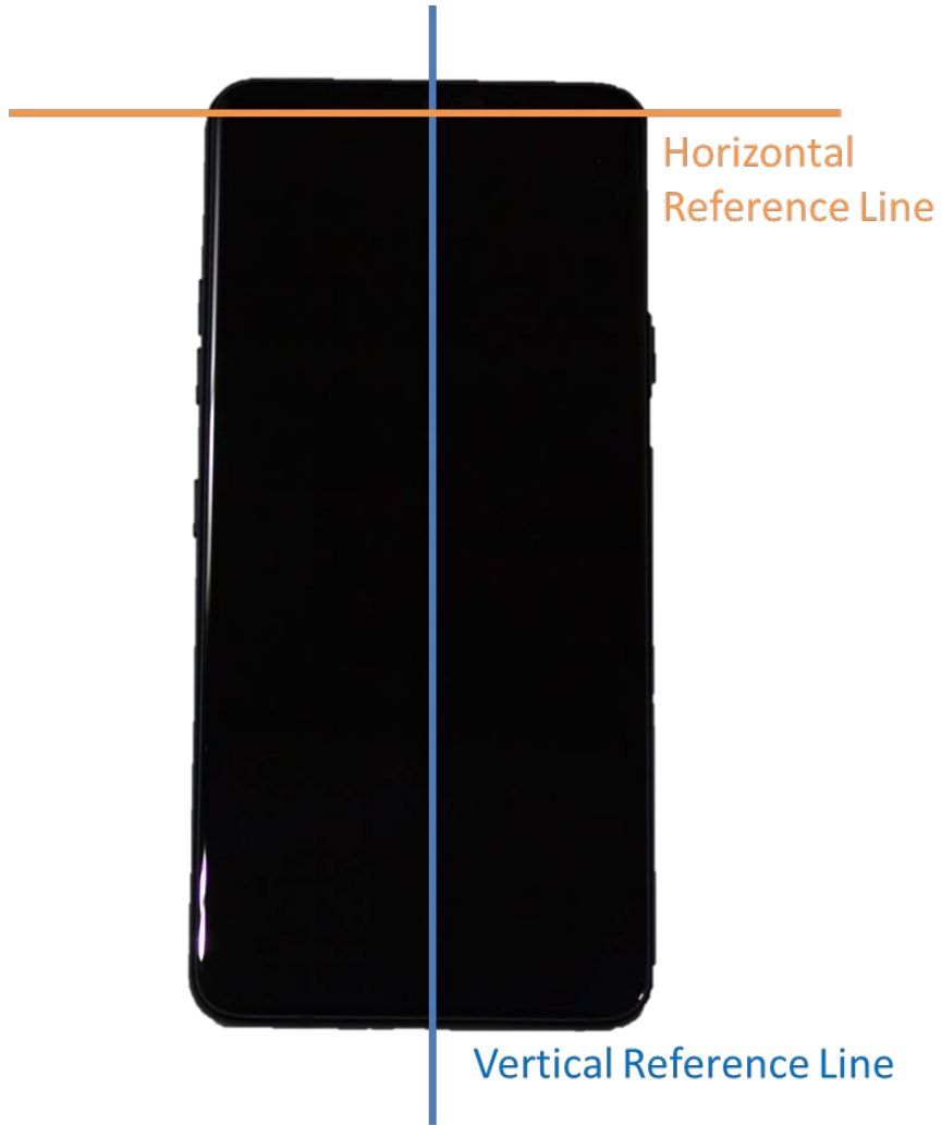
SAR Test Setup Photo 19 – Horizontal and Vertical Reference Lines
