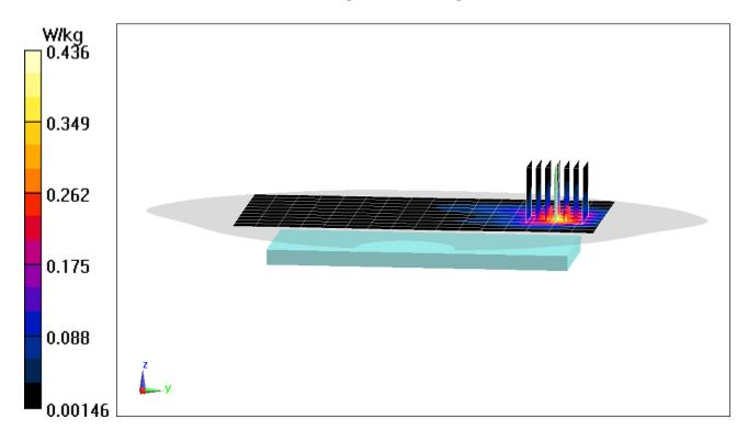
DUT: ZNFQ910QM; Type: Portable Handset; Serial: 19850
