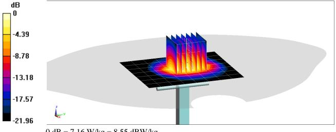
**DUT: Dipole 2600 MHz; Type: D2600V2; Serial: 1071**
