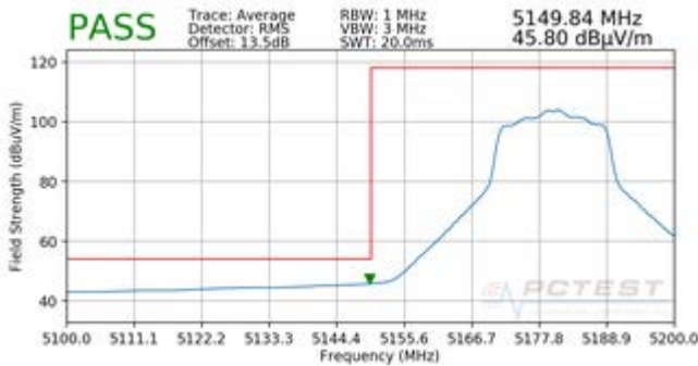
Plot 7-193. Radiated Lower Band Edge Plot SISO ANT2 (Average – UNII Band 1)
