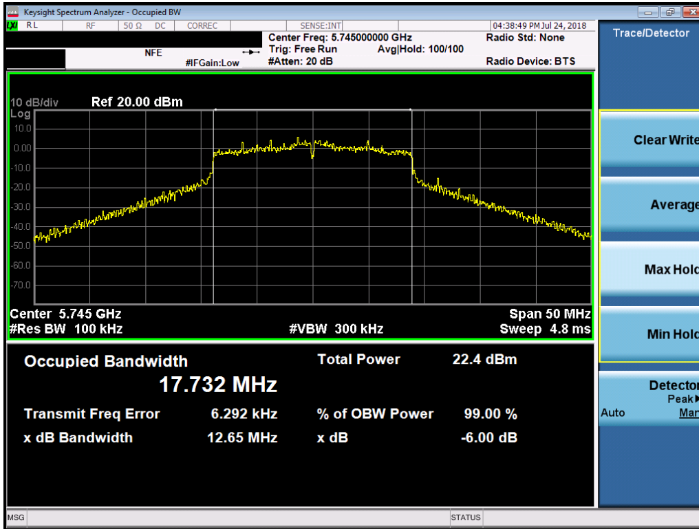
Plot 7-64. 6dB Bandwidth Plot SISO ANT1 (20MHz BW 802.11n (UNII Band 3) – Ch. 149)
