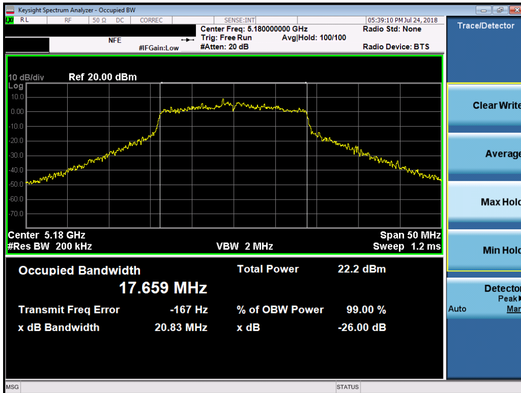
Plot 7-34. 26dB Bandwidth Plot SISO ANT2 (20MHz BW 802.11n (UNII Band 1) – Ch. 36)
