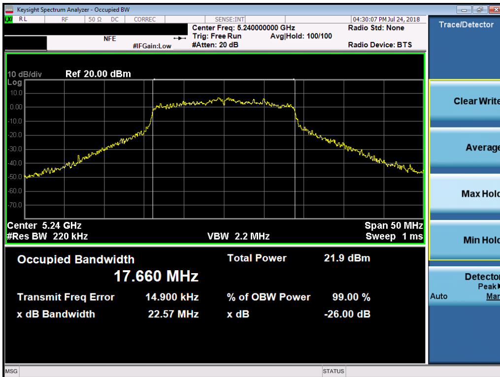
Plot 7-6. 26dB Bandwidth Plot SISO ANT1 (20MHz BW 802.11n (UNII Band 1) – Ch. 48)
