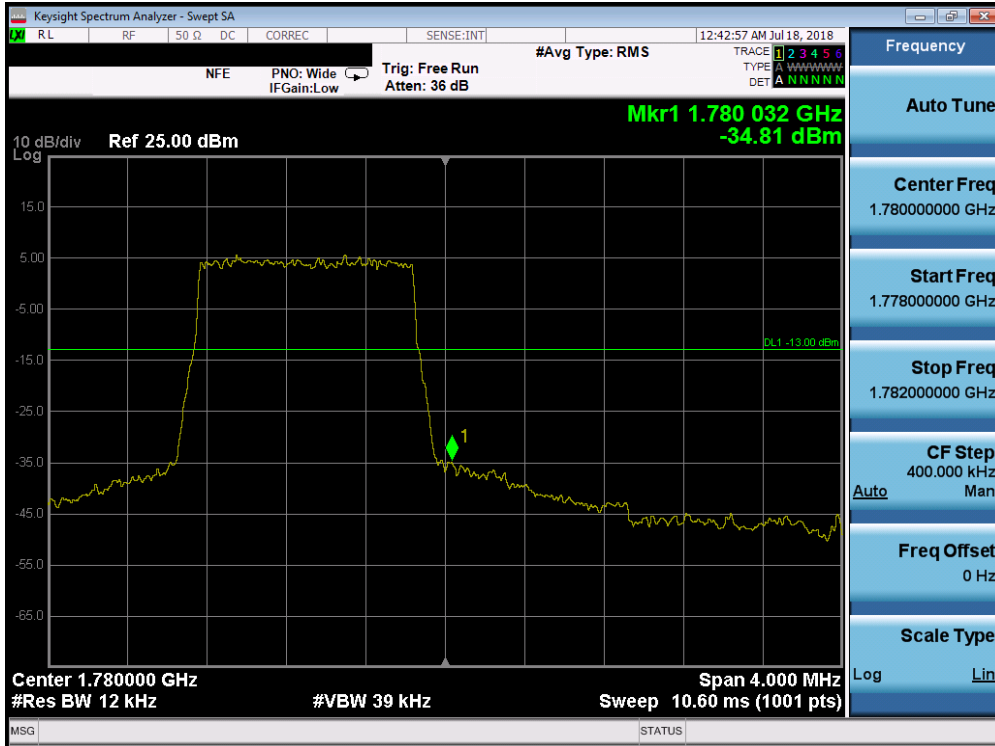
Plot 7-193. Upper Band Edge Plot (Band 66 - 1.4MHz QPSK - Full RB Configuration)
