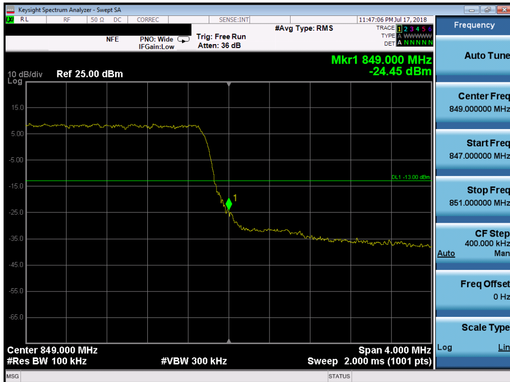
Plot 7-186. Upper Band Edge Plot (Band 26/5 - 5.0MHz QPSK - Full RB Configuration)
