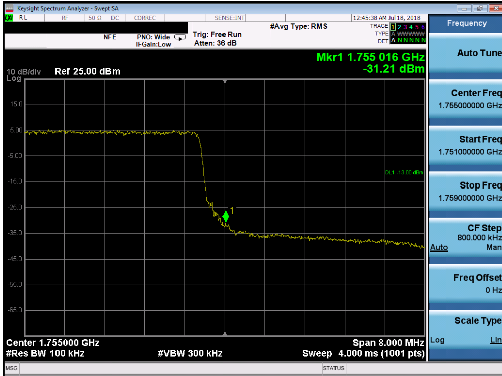
Plot 7-209. Upper Band Edge Plot (Band 4 - 10.0MHz QPSK - Full RB Configuration)
