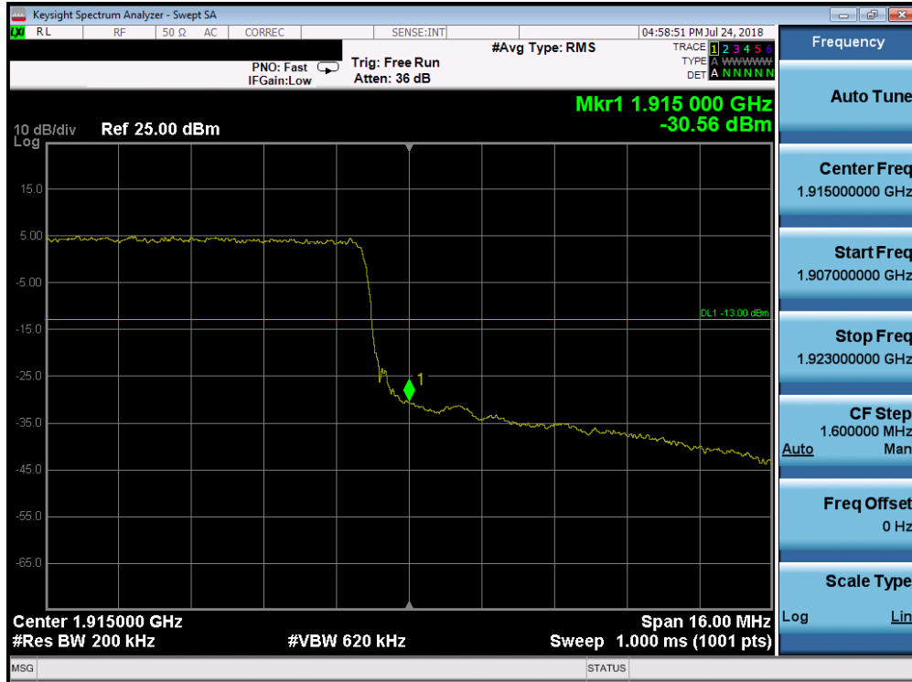
Plot 7-259. Upper Band Edge Plot (Band 25 - 20.0MHz QPSK - Full RB Configuration)
