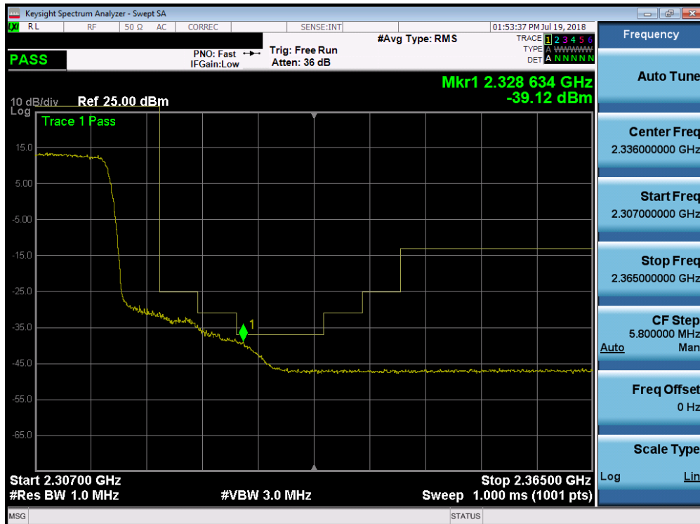
Plot 7-268. Upper Extended Band Edge Plot (Band 30 - 10.0MHz QPSK - Full RB Configuration)
