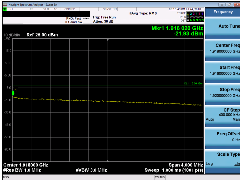
Plot 7-248. Upper Extended Band Edge Plot (Band 25 - 10.0MHz QPSK - Full RB Configuration)
