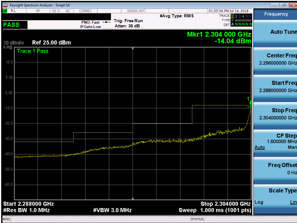
Plot 7-262. Lower Extended Band Edge Plot (Band 30 - 5.0MHz QPSK - Full RB Configuration)
