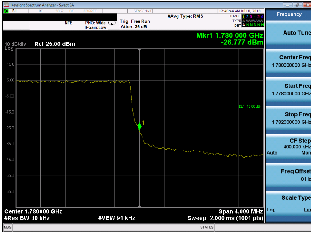
Plot 7-199. Upper Band Edge Plot (Band 66 - 3.0MHz QPSK - Full RB Configuration)
