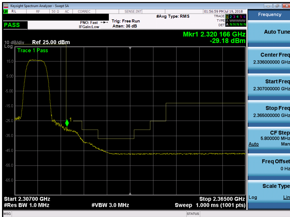
Plot 7-264. Upper Extended Band Edge Plot (Band 30 - 5.0MHz QPSK - Full RB Configuration)
