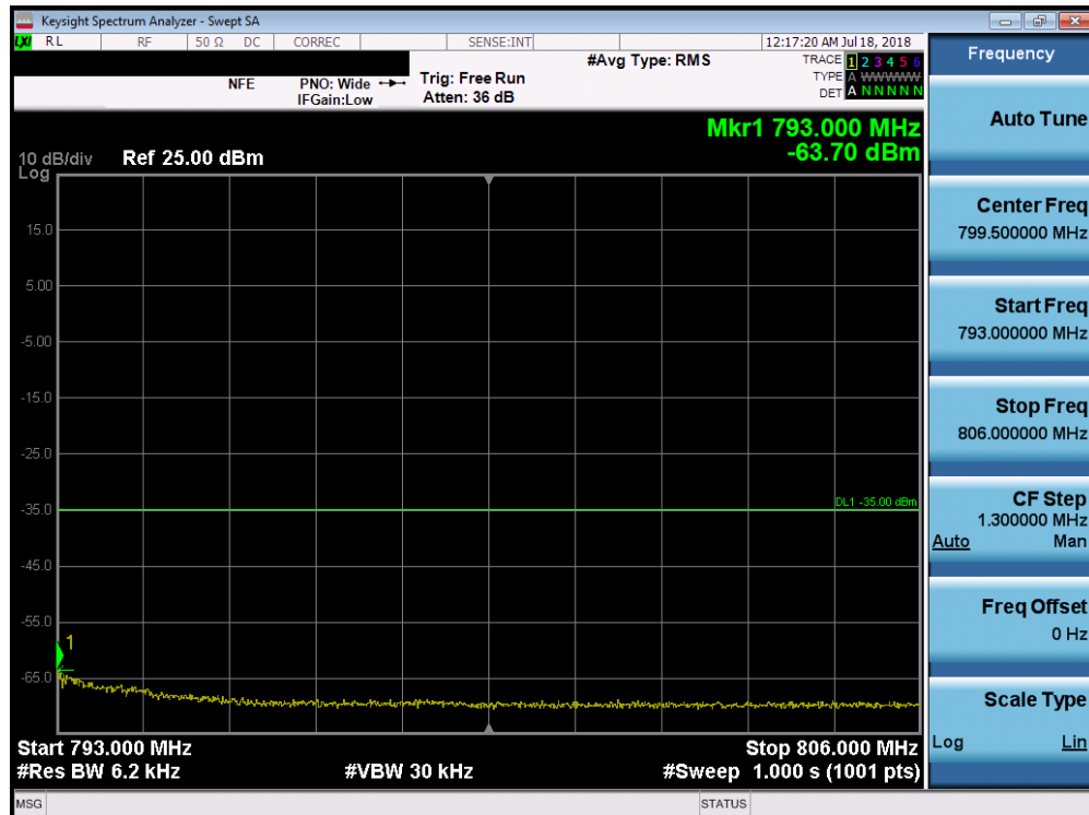
Plot 7-176. Upper Emission Mask Plot (Band 13 - 5.0MHz QPSK - Full RB Configuration)
