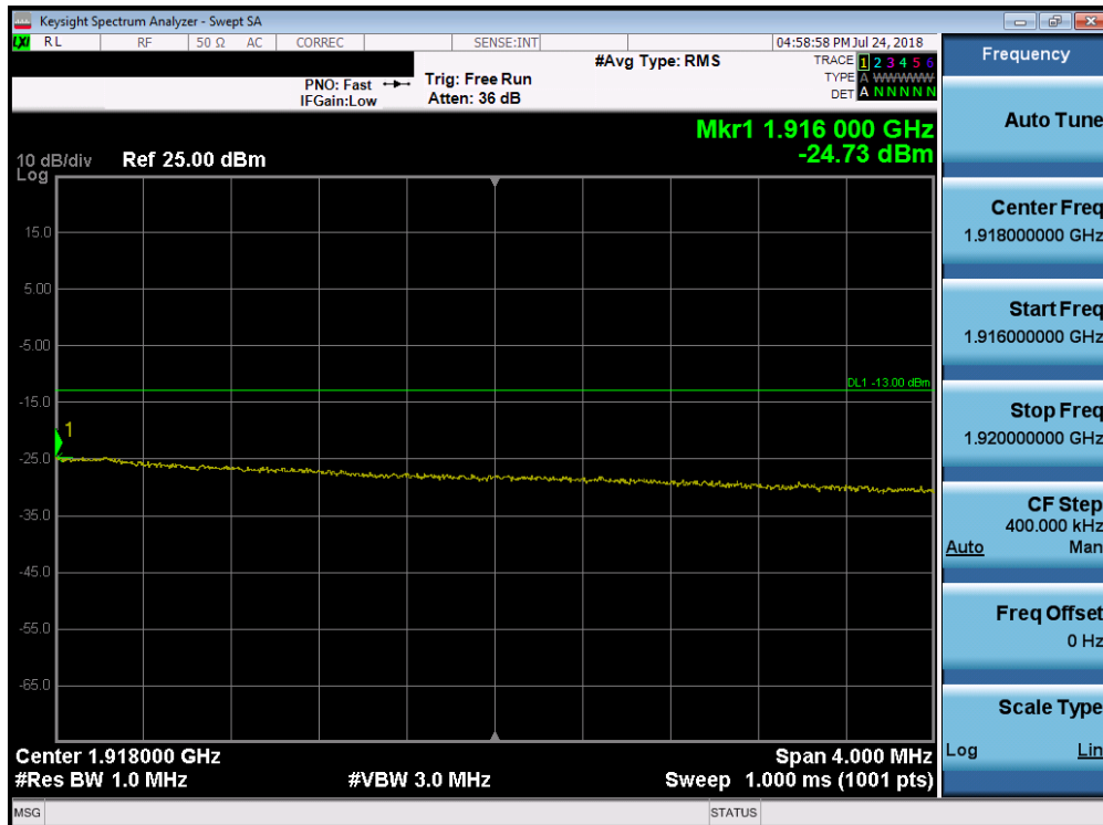
Plot 7-260. Upper Extended Band Edge Plot (Band 25 - 20.0MHz QPSK - Full RB Configuration)
