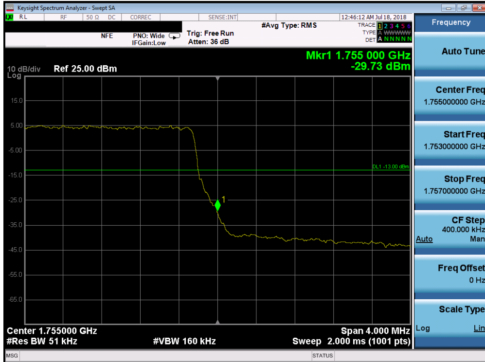
Plot 7-203. Upper Band Edge Plot (Band 4 - 5.0MHz QPSK - Full RB Configuration)
