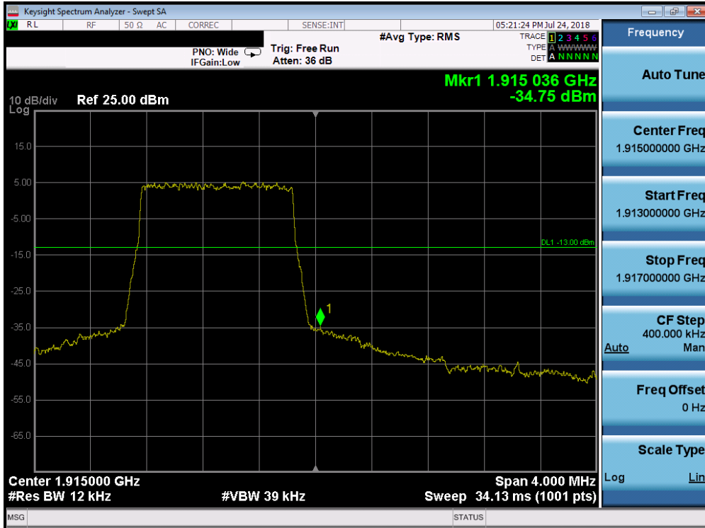
Plot 7-229. Upper Band Edge Plot (Band 25 - 1.4MHz QPSK - Full RB Configuration)
