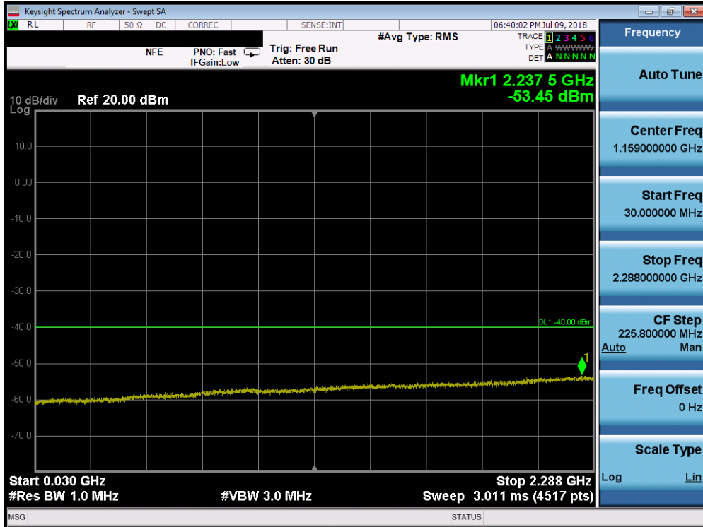
Plot 7-142. Conducted Spurious Plot (Band 30 - 5.0MHz QPSK - RB Size 1, RB Offset 0 – High Channel)
