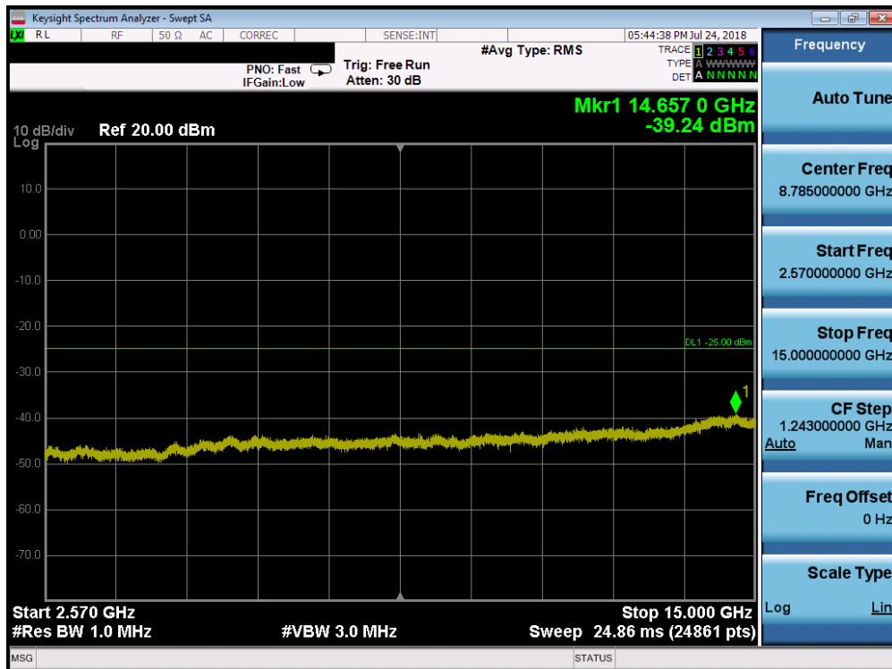
Plot 7-146. Conducted Spurious Plot (Band 7 - 20.0MHz QPSK - RB Size 1, RB Offset 0 - Low Channel)
