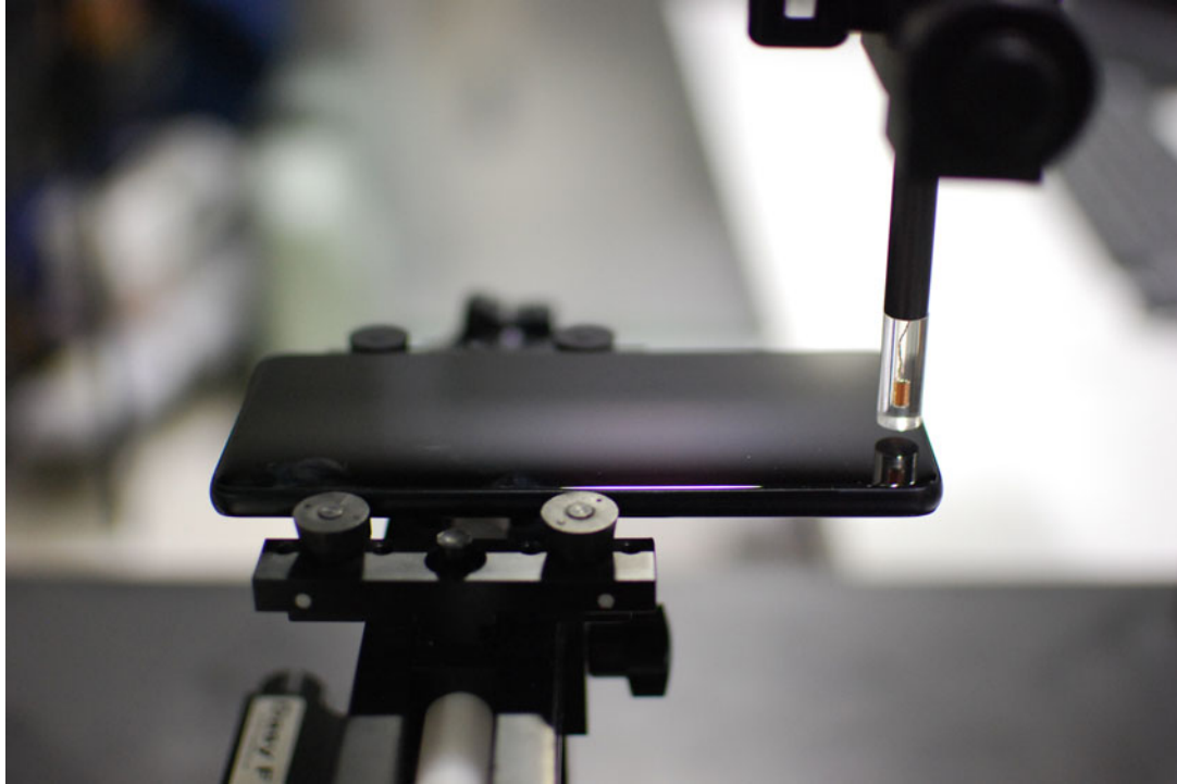
Figure 16-1 Test Setup for Wireless Device
