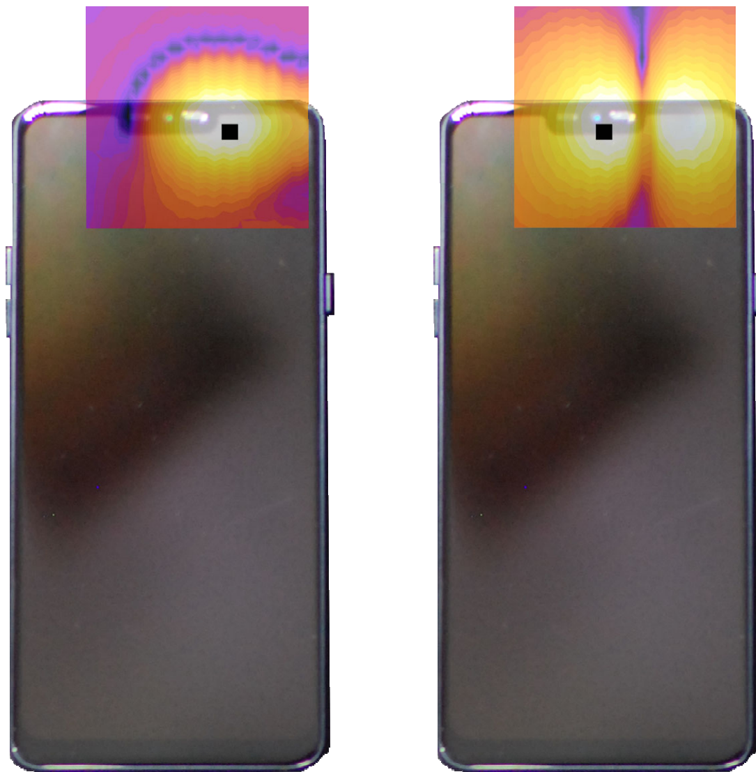
Figure 16-3 T-Coil Scan Overlay Magnetic Field Distributions
