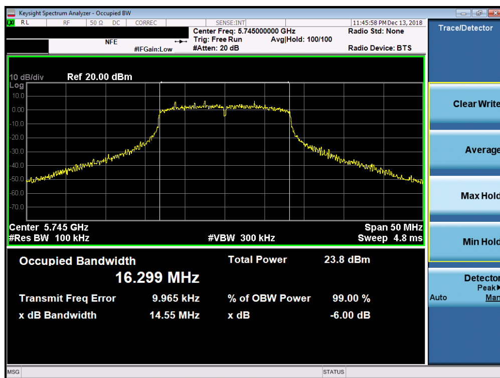
Plot 7-61. 6dB Bandwidth Plot SISO ANT1 (802.11a (UNII Band 3) - Ch. 149)
