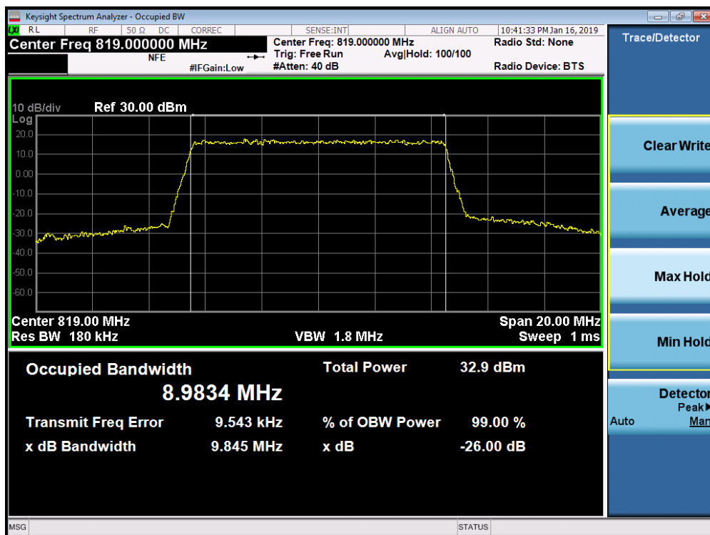
Plot 7-12. Occupied Bandwidth Plot (LTE Band 26, 10MHz QPSK – RB Size 50)
