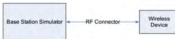
Figure 9.1 Power Measurement Setup
