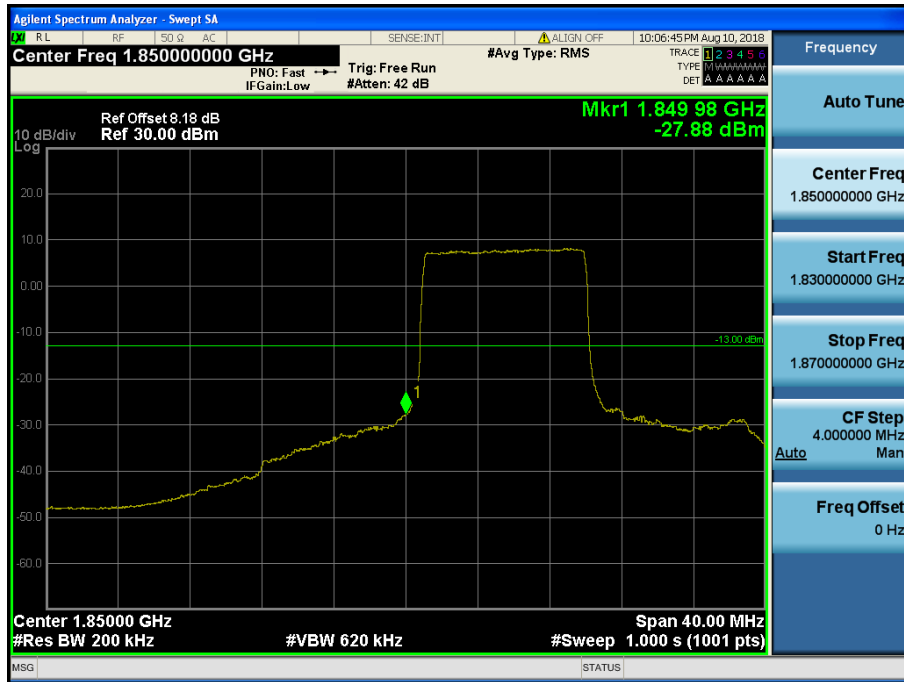
LTE Band 2 / 20MHz / QPSK - RB Size/Offset (50/0)
