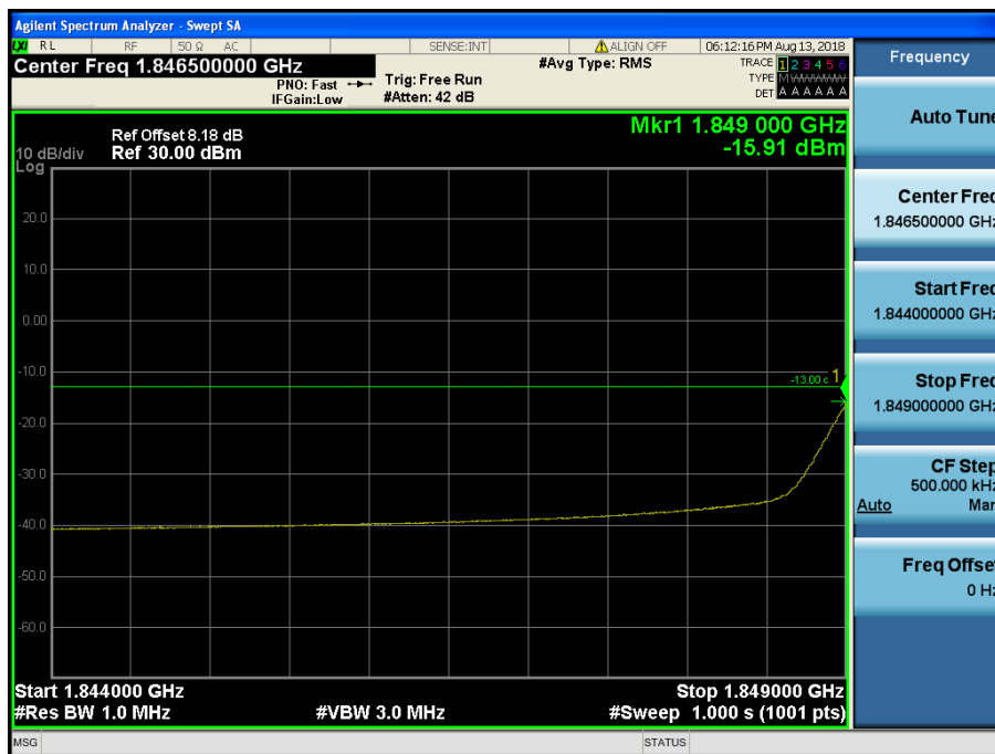
LTE Band 2 / 1.4MHz / 64QAM - RB Size/Offset (3/2)
