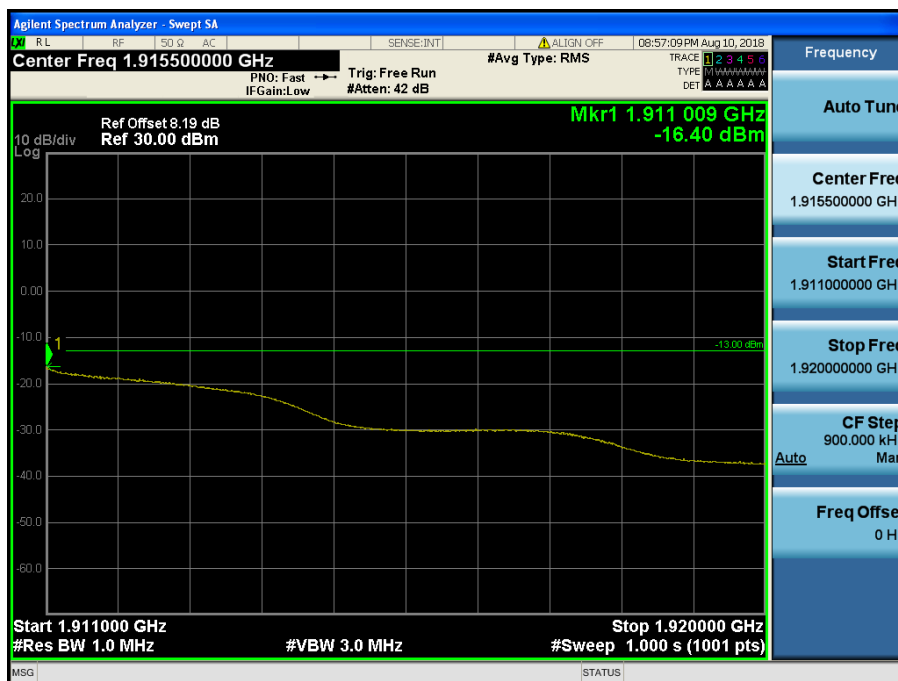
LTE Band 2 / 10MHz / QPSK - RB Size/Offset (25/25)
