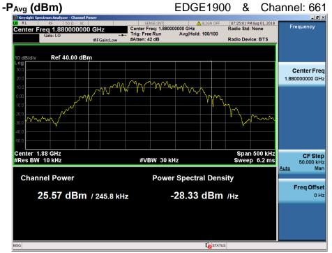
PAPR (dB) =  $P_{Pk}$  (dBm) -  $P_{Avg}$  (dBm) = 29.05 dBm - 25.57 dBm = 3.48 dB
