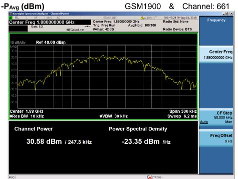
$PAPR (dB) = P_{Pk} (dBm) - P_{Avg} (dBm) = 30.84 dBm - 30.58 dBm = 0.26 dB$
