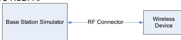
Figure 9-3 Power Measurement Setup
