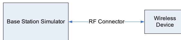
Figure 9-4 Power Measurement Setup
