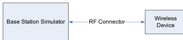
Figure 9-2 Power Measurement Setup
