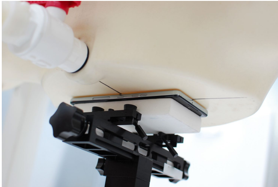
SAR Test Setup Photo 6 – Back Side at 1 mm
