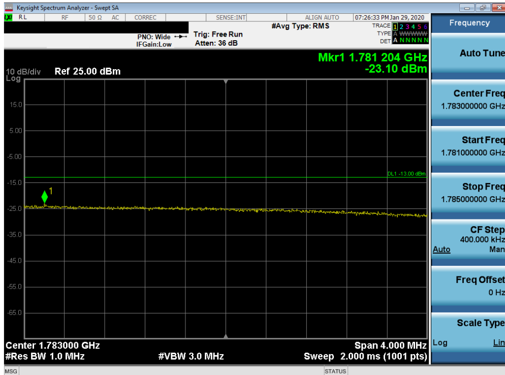
Plot 7-214. Upper Extended Band Edge Plot (Band 66 - 15.0MHz QPSK - Full RB Configuration)
