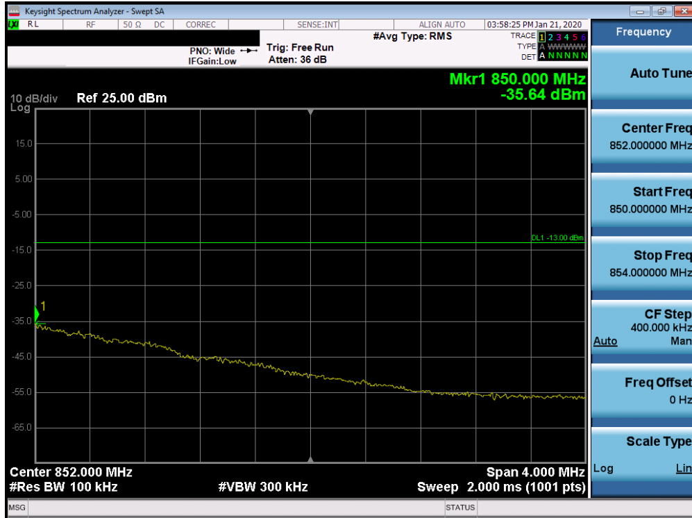
Plot 7-176. Upper Extended Band Edge Plot (Band 26/5 - 1.4MHz QPSK - Full RB Configuration)
