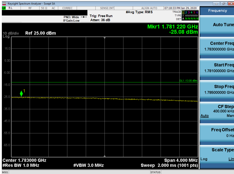
Plot 7-220. Upper Extended Band Edge Plot (Band 66 - 20.0MHz QPSK - Full RB Configuration)
