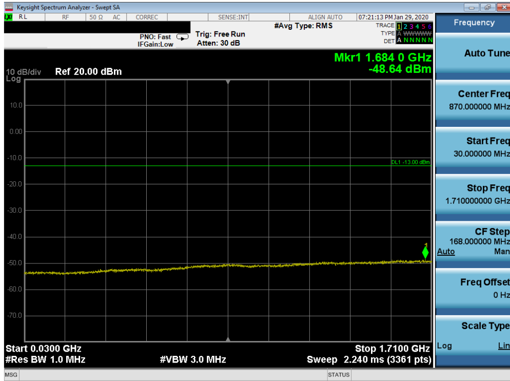
Plot 7-124. Conducted Spurious Plot (Band 66/4 - 15.0MHz QPSK - RB Size 1, RB Offset 0 - Mid Channel)
