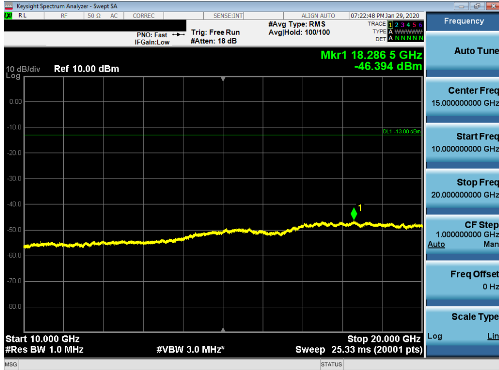
Plot 7-126. Conducted Spurious Plot (Band 66/4 - 15.0MHz QPSK - RB Size 1, RB Offset 0 - Mid Channel)
