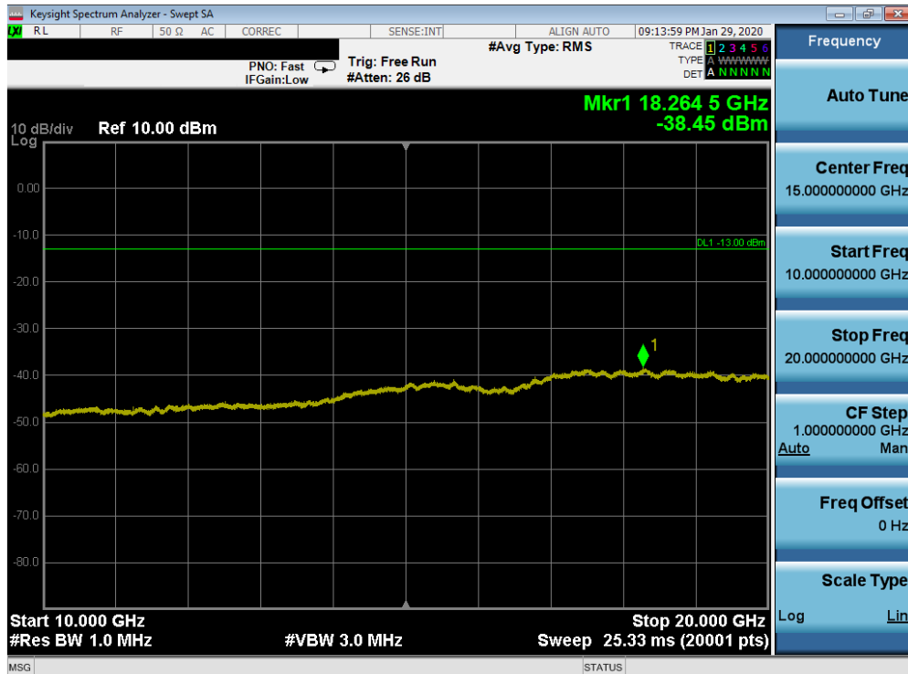
Plot 7-141. Conducted Spurious Plot (Band 25/2 - 20.0MHz QPSK - RB Size 1, RB Offset 0 - Mid Channel)
