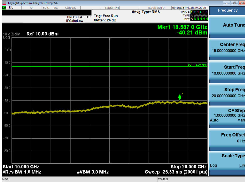
Plot 7-138. Conducted Spurious Plot (Band 25/2 - 20.0MHz QPSK - RB Size 1, RB Offset 0 - Low Channel)
