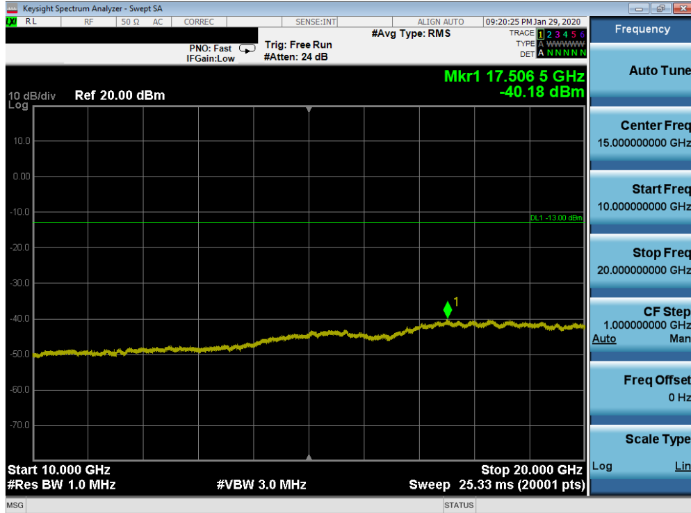
Plot 7-144. Conducted Spurious Plot (Band 25/2 - 20.0MHz QPSK - RB Size 1, RB Offset 0 - High Channel)
