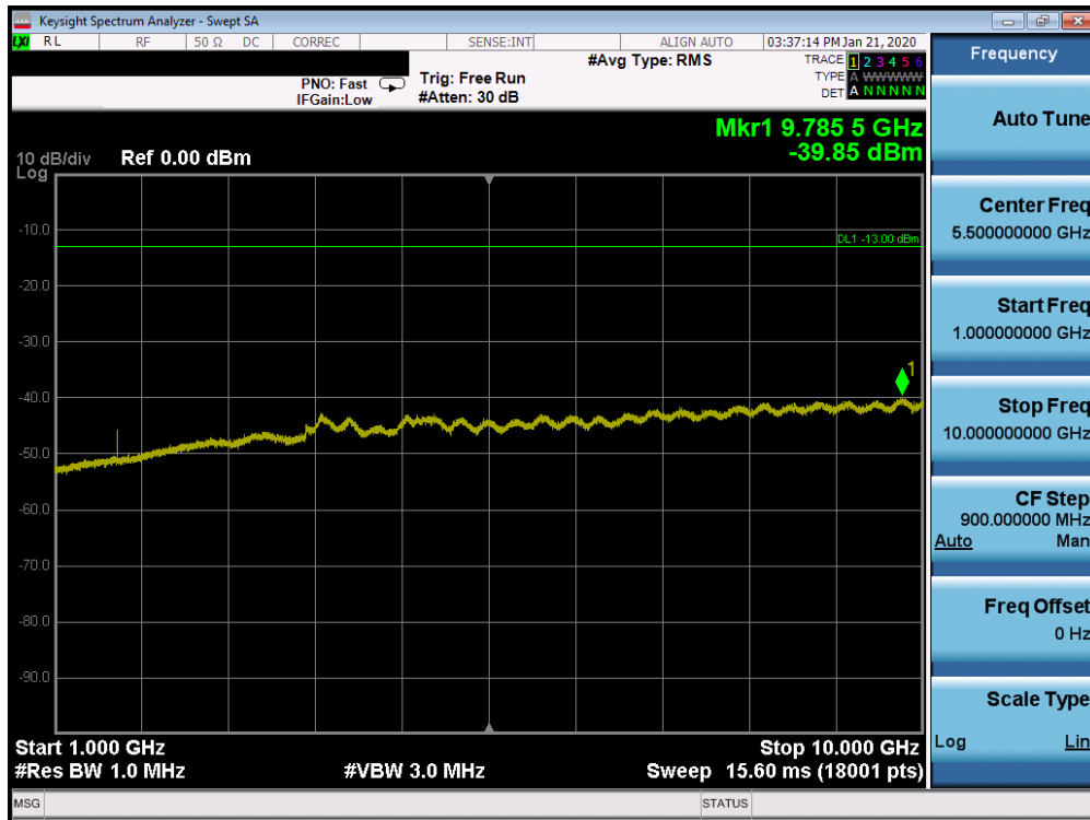
Plot 7-117. Conducted Spurious Plot (Band 26 - 10.0MHz QPSK - RB Size 1, RB Offset 0 - Low Channel)
