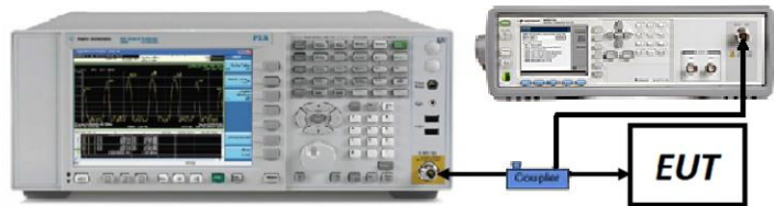
Figure 7-2. Test Instrument & Measurement Setup
