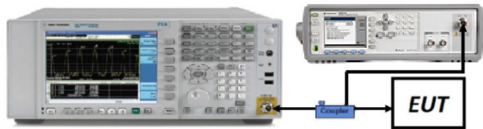
Figure 7-4. Test Instrument & Measurement Setup
