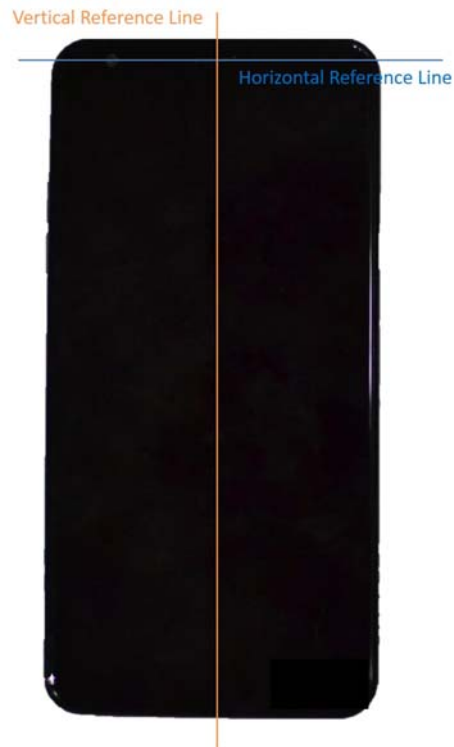
SAR Test Setup Photo 16 – Horizontal and Vertical Reference Lines
