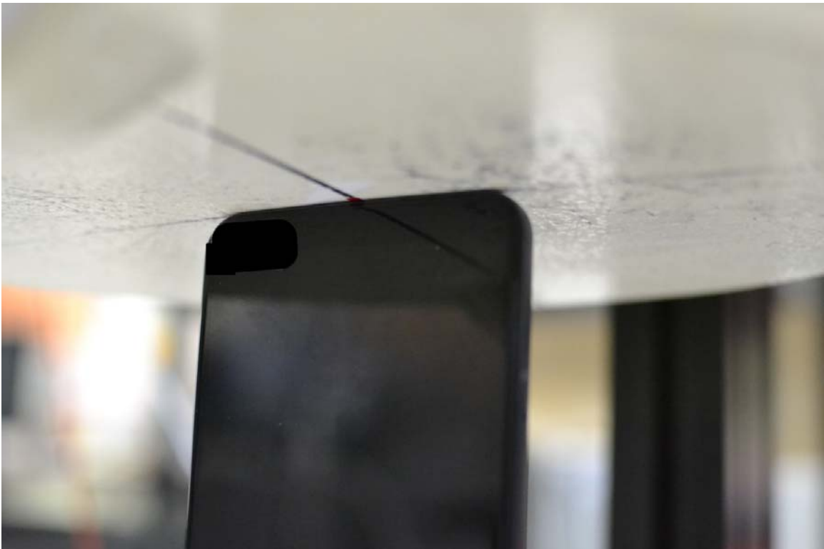
SAR Test Setup Photo 12 – Bottom Edge at 0.0cm
