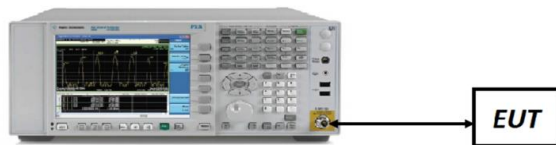
Figure 7-5. Test Instrument & Measurement Setup
