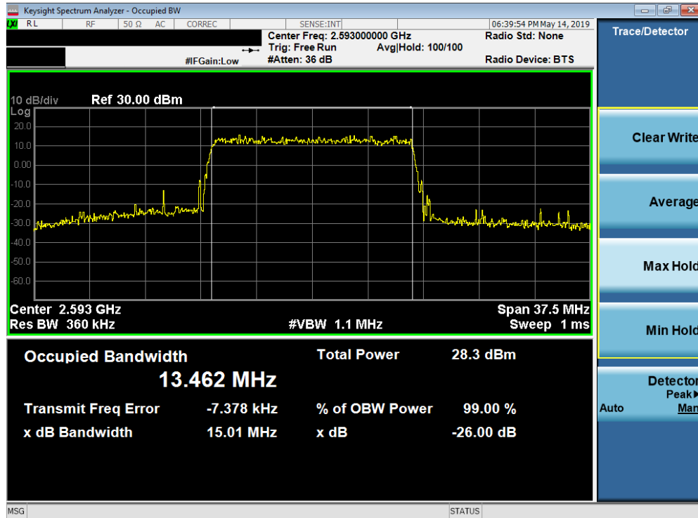
Plot 7-90. Occupied Bandwidth Plot (Band 41 - 15.0MHz 64-QAM - Full RB Configuration)
