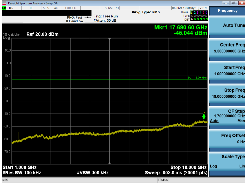
Plot 7-26. Conducted Spurious Plot (LTE Band 26, 15MHz QPSK – RB Size 1, RB Offset 0)
