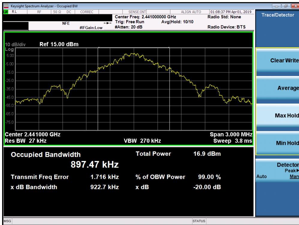
Plot 7-2. 20dB Bandwidth Plot (Bluetooth, 1Mbps – Ch. 39)
