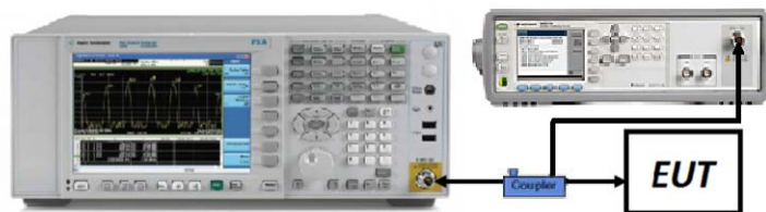
Figure 7-1. Test Instrument & Measurement Setup
