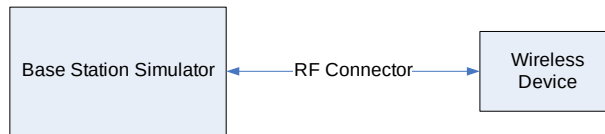
Figure 9-2 Power Measurement Setup
