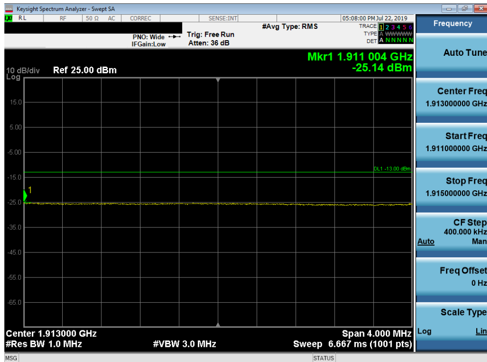
Plot 7-159. Upper Extended Band Edge Plot (Band 2 - 20.0MHz QPSK - Full RB Configuration)
