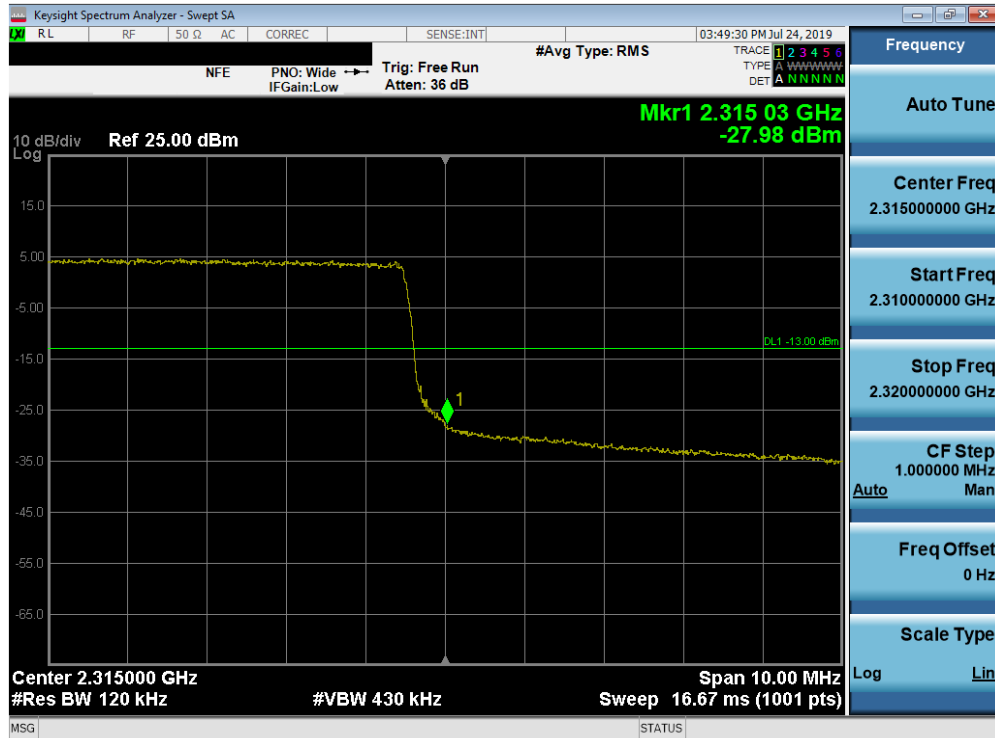
Plot 7-166. Upper Band Edge Plot (Band 30 - 10.0MHz QPSK - Full RB Configuration)
