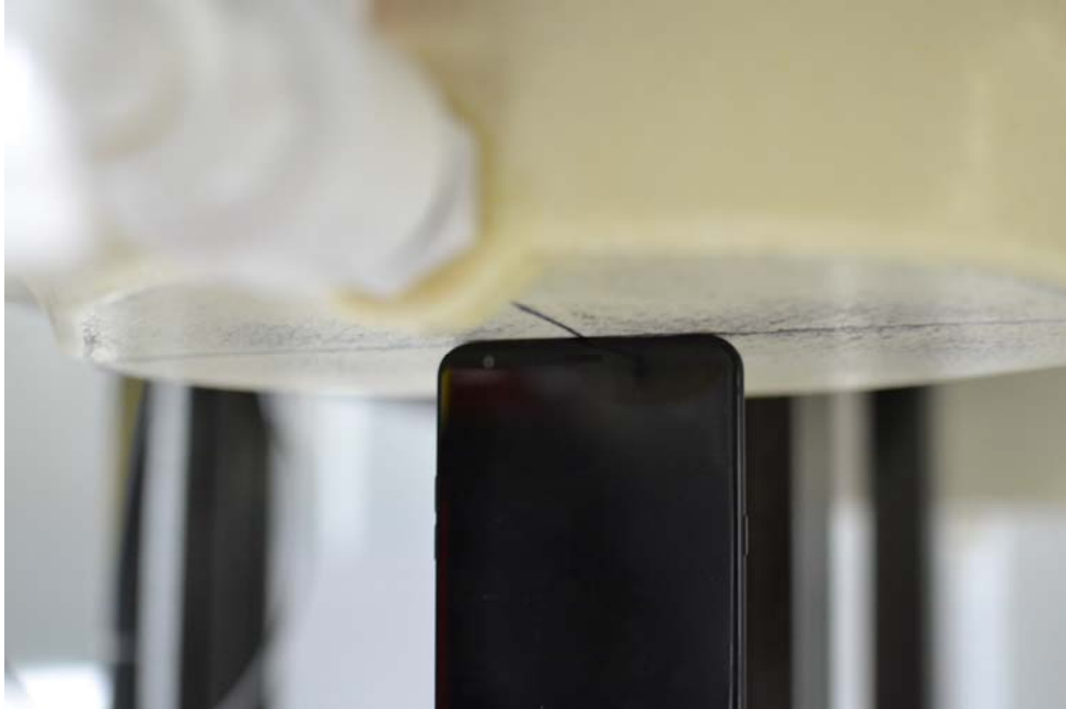
SAR Test Setup Photo 14: Top at 0.0 cm
