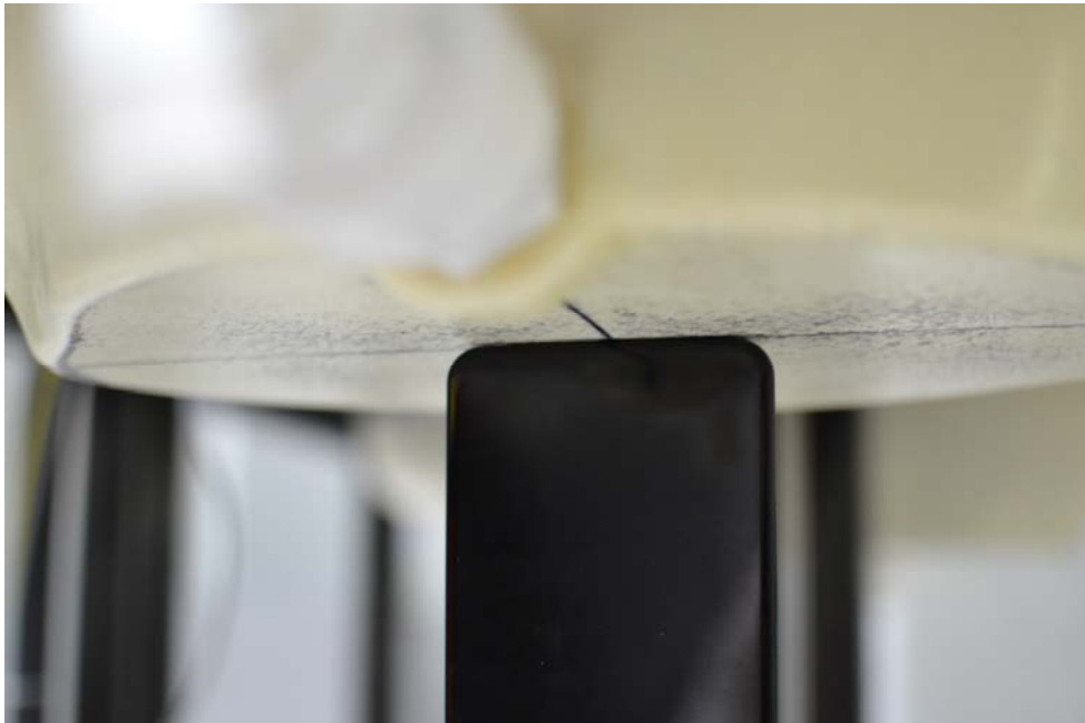
SAR Test Setup Photo 15: Bottom at 0.0 cm
