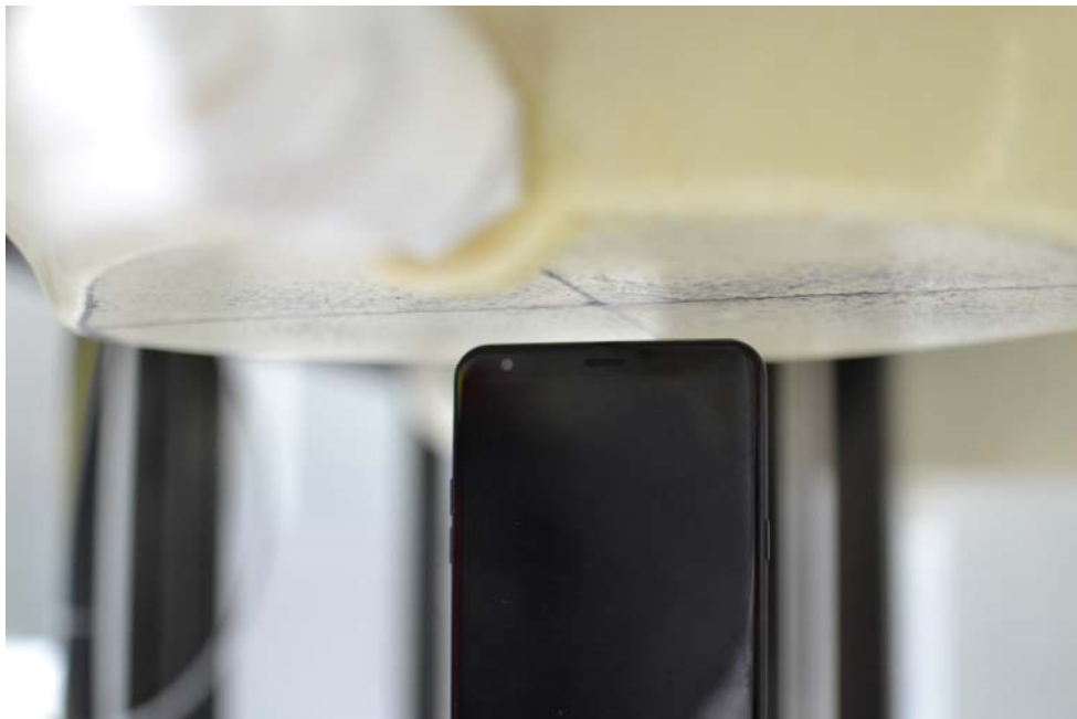
SAR Test Setup Photo 7: Top at 1.0 cm
