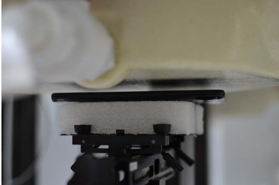
SAR Test Setup Photo 6: Front at 1.0 cm
