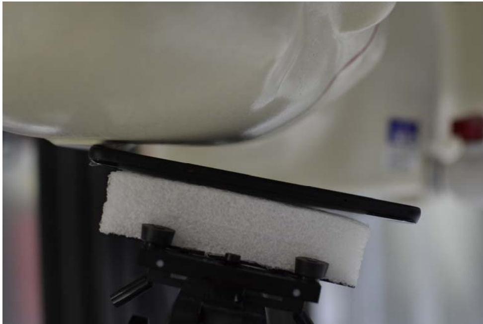
SAR Test Setup Photo 2: Right Tilt
