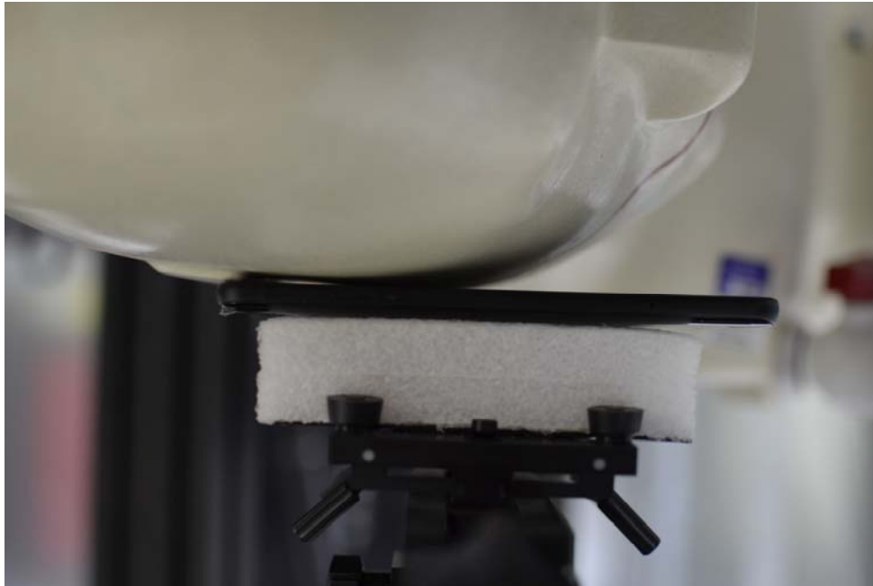
SAR Test Setup Photo 1: Right Cheek
