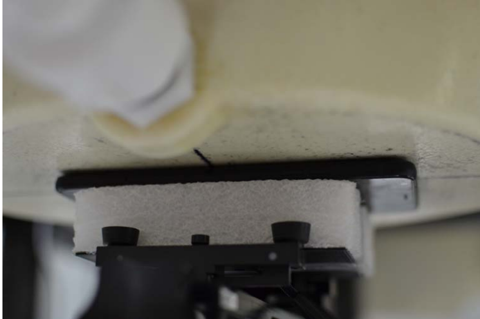
SAR Test Setup Photo 10: Back at 0.0 cm
