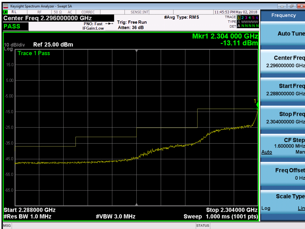
Plot 7-197. Lower Extended Band Edge Plot (Band 30 - 5.0MHz QPSK - Full RB Configuration)
