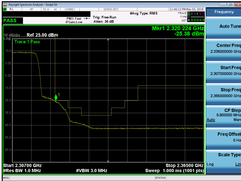
Plot 7-203. Upper Extended Band Edge Plot (Band 30 - 10.0MHz QPSK - Full RB Configuration)
