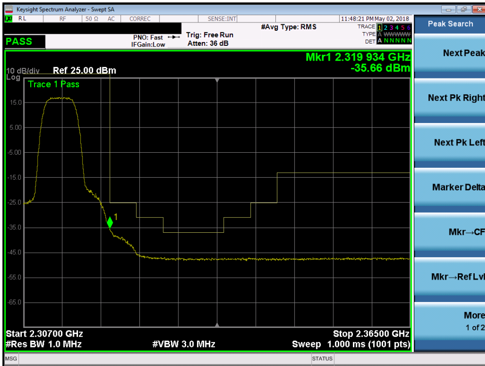
Plot 7-199. Upper Extended Band Edge Plot (Band 30 - 5.0MHz QPSK - Full RB Configuration)
