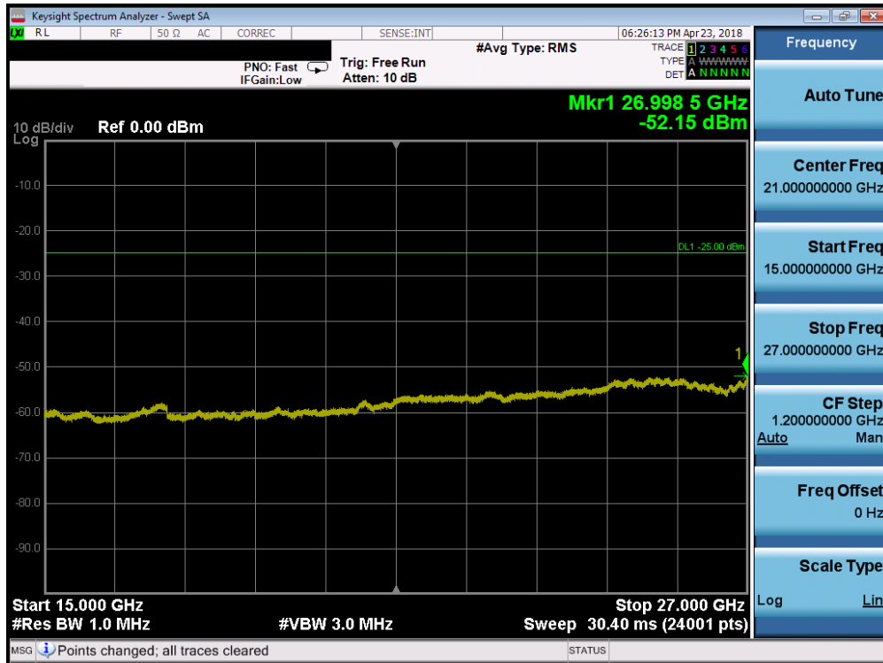
Plot 7-113. Conducted Spurious Plot (Band 7 - 20.0MHz QPSK - RB Size 1, RB Offset 0 - High Channel)
