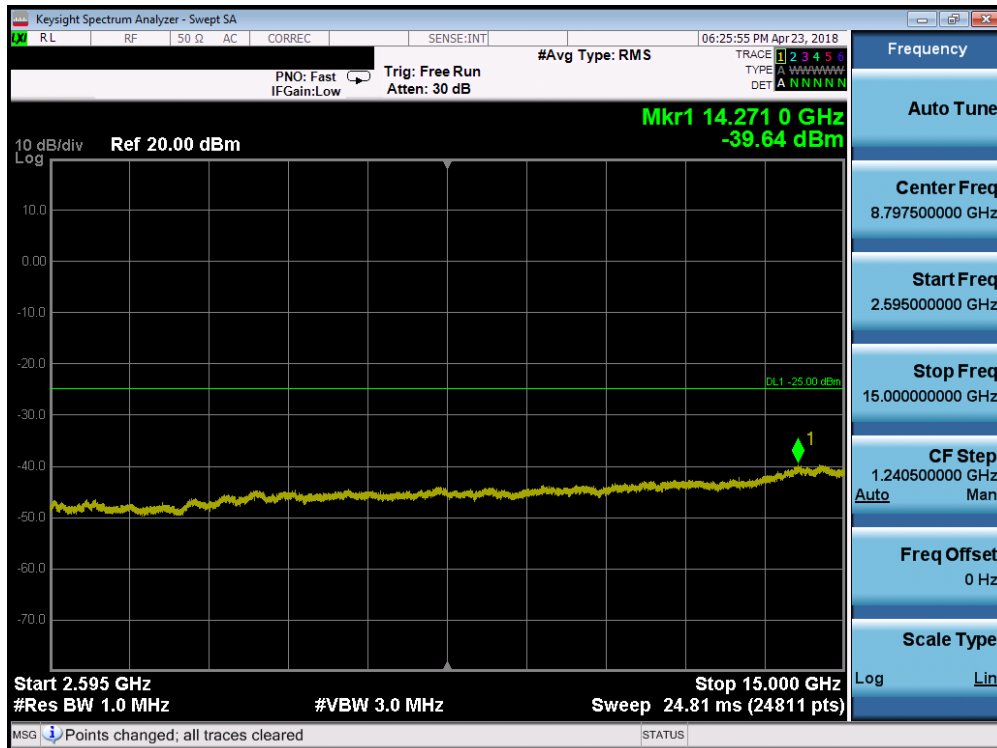
Plot 7-112. Conducted Spurious Plot (Band 7 - 20.0MHz QPSK - RB Size 1, RB Offset 0 - High Channel)
