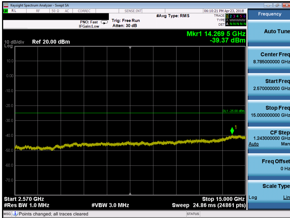
Plot 7-109. Conducted Spurious Plot (Band 7 - 20.0MHz QPSK - RB Size 1, RB Offset 0 - Mid Channel)
