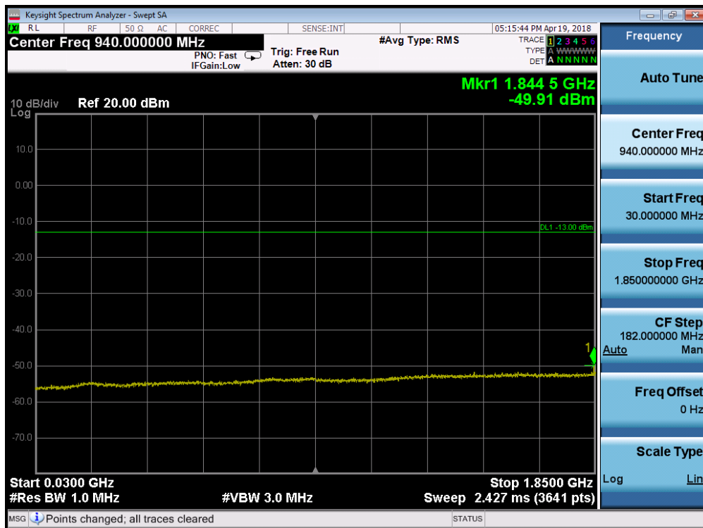
Plot 7-90. Conducted Spurious Plot (Band 25/2 - 20.0MHz QPSK - RB Size 1, RB Offset 0 - Mid Channel)
