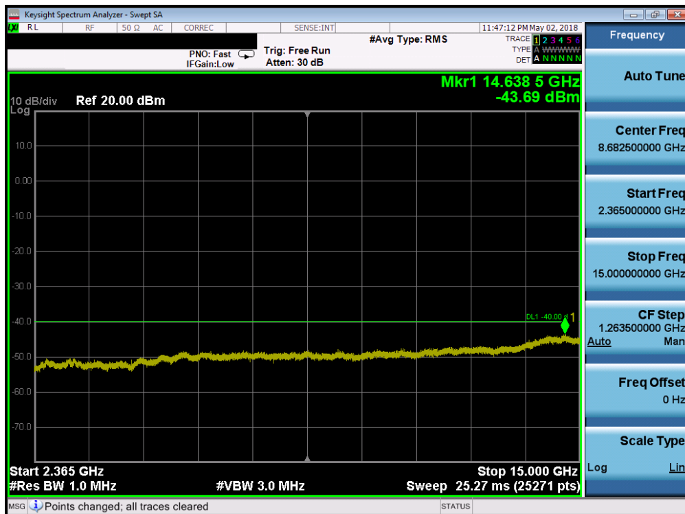
Plot 7-103. Conducted Spurious Plot (Band 30 - 5.0MHz QPSK - RB Size 1, RB Offset 0 - High Channel)
