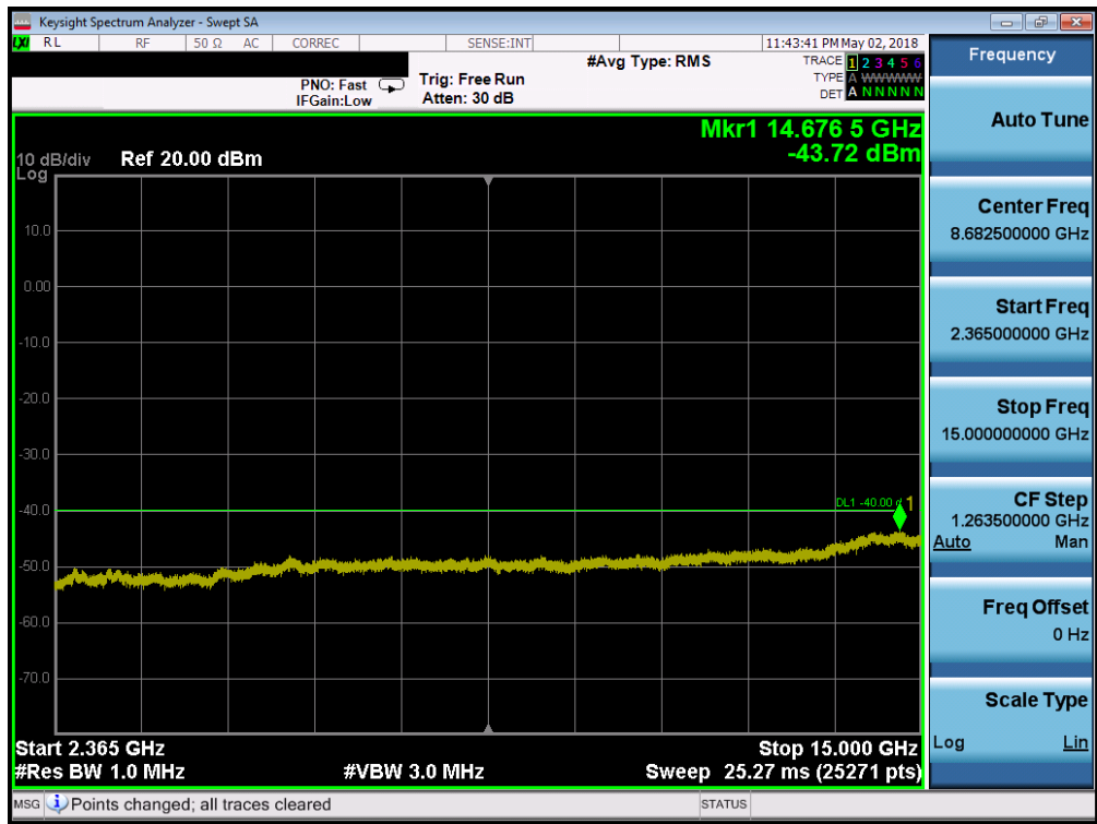
Plot 7-100. Conducted Spurious Plot (Band 30 - 5.0MHz QPSK - RB Size 1, RB Offset 0 - Mid Channel)
