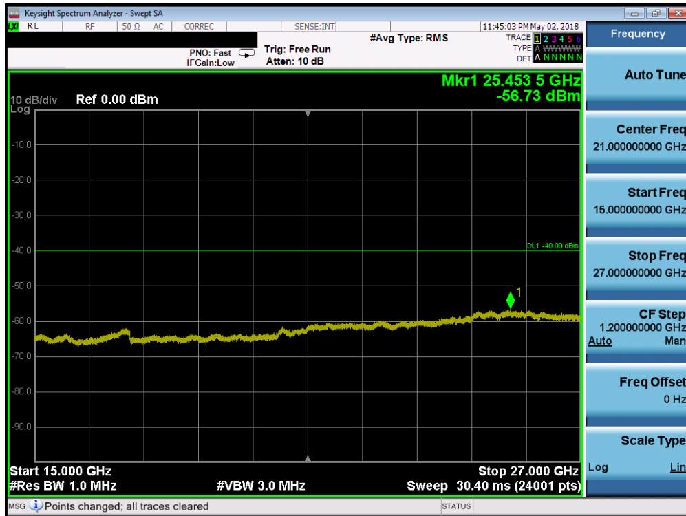
Plot 7-98. Conducted Spurious Plot (Band 30 - 5.0MHz QPSK - RB Size 1, RB Offset 0 - Low Channel)
