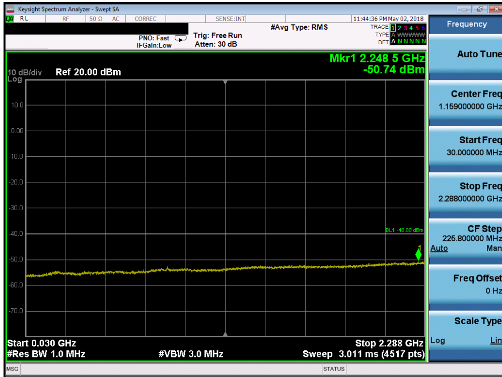
Plot 7-96. Conducted Spurious Plot (Band 30 - 5.0MHz QPSK - RB Size 1, RB Offset 0 - Low Channel)
