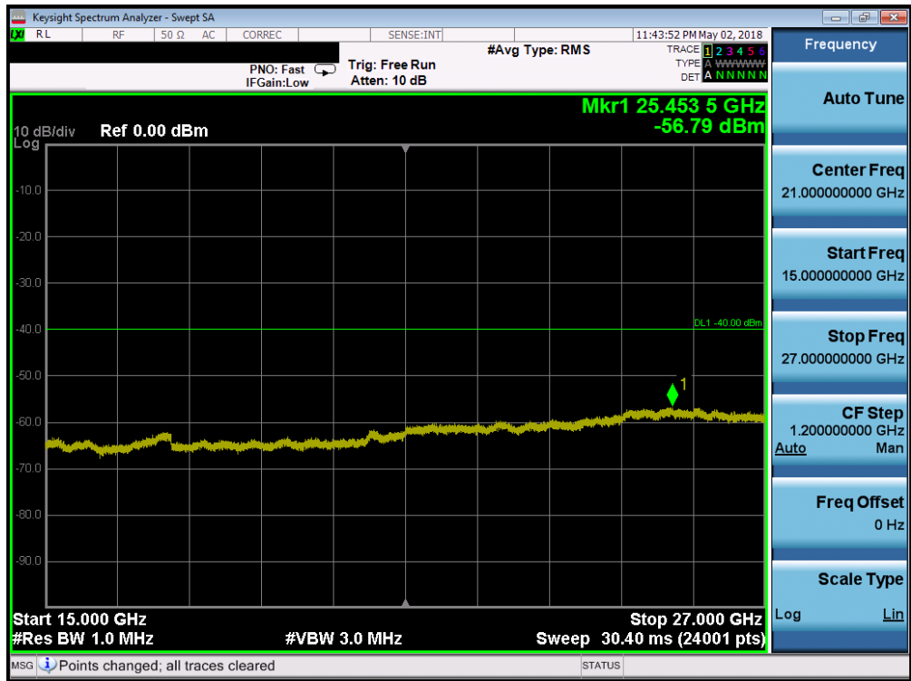
Plot 7-101. Conducted Spurious Plot (Band 30 - 5.0MHz QPSK - RB Size 1, RB Offset 0 - Mid Channel)
