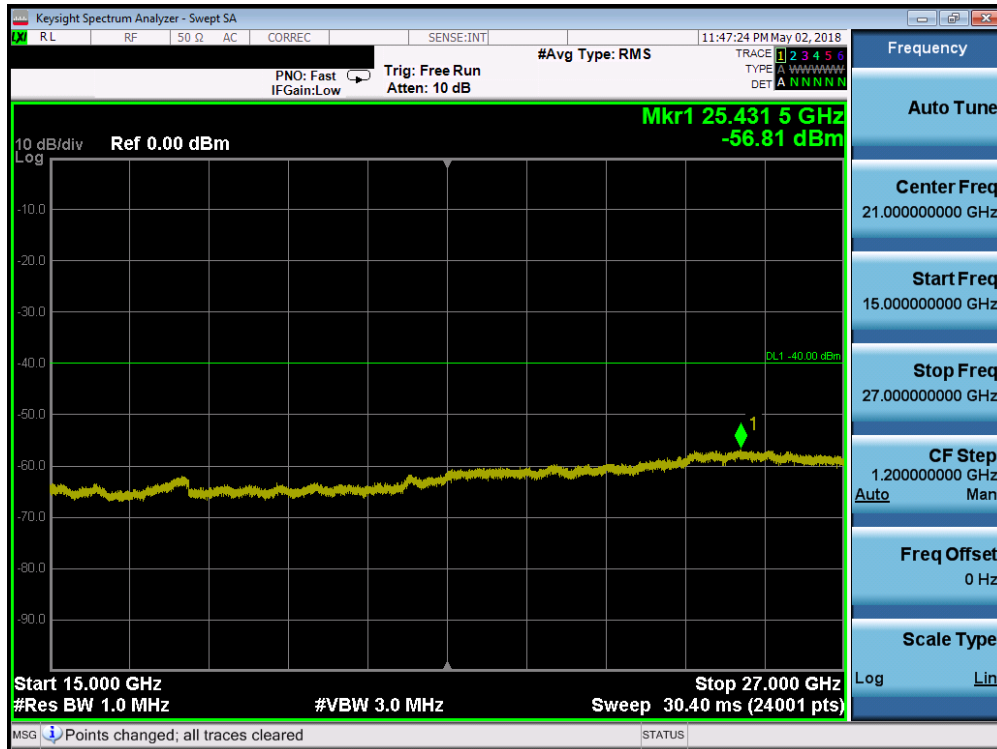
Plot 7-104. Conducted Spurious Plot (Band 30 - 5.0MHz QPSK - RB Size 1, RB Offset 0 - High Channel)
