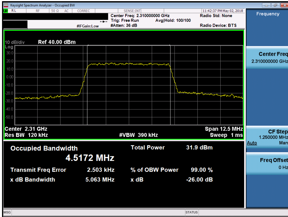
Plot 7-45. Occupied Bandwidth Plot (Band 30 - 5.0MHz QPSK - Full RB Configuration)
